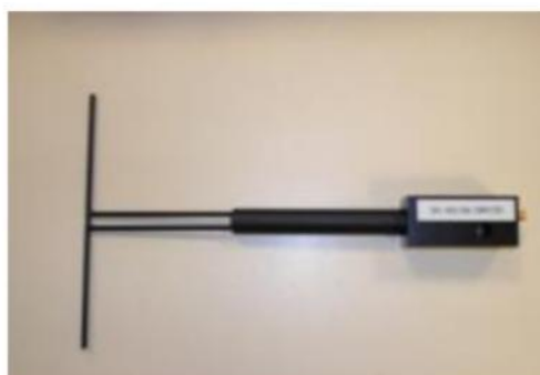
Figure 1 – Satimo COMOSAR Validation Dipole
