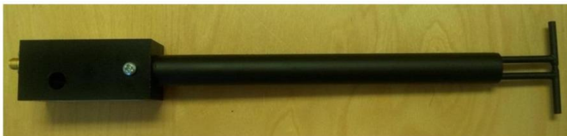
Figure 1 – MVG COMOSAR Validation Dipole
