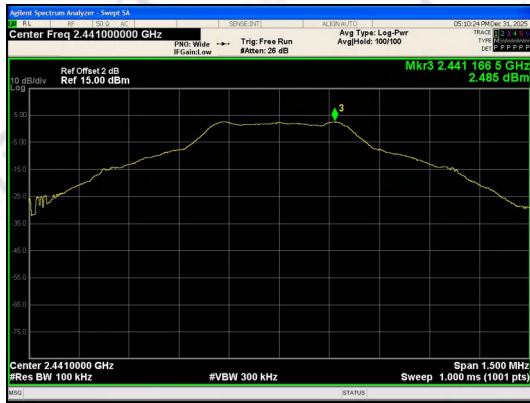
In-Band Reference Level GFSK_DH5_Channel 39
