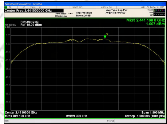
In-Band Reference Level \pi/4 DQPSK_2-DH5_Channel 39
