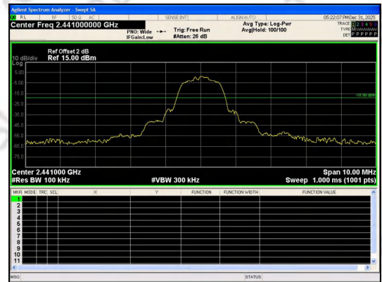
Out Of Band Emission \pi/4 DQPSK_2-DH5_Channel 39
