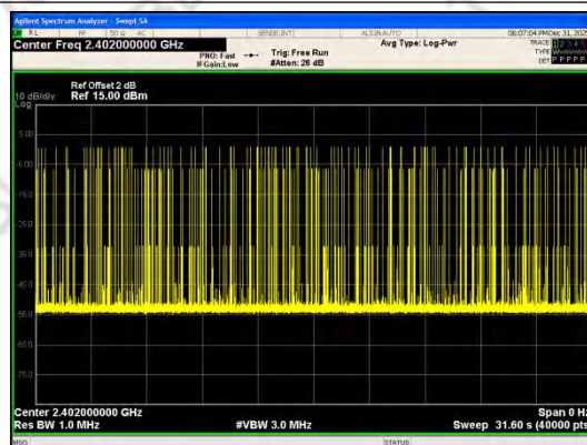
Number of Pulses in 31.6 seconds GFSK DH5
