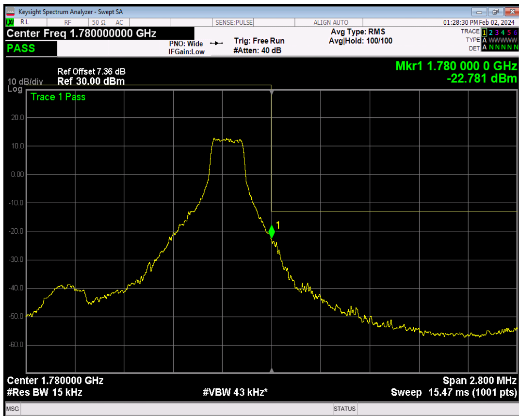
Band66 16QAM BW=1.4MHz Channel=132665 RB Size=6 Position=#0
