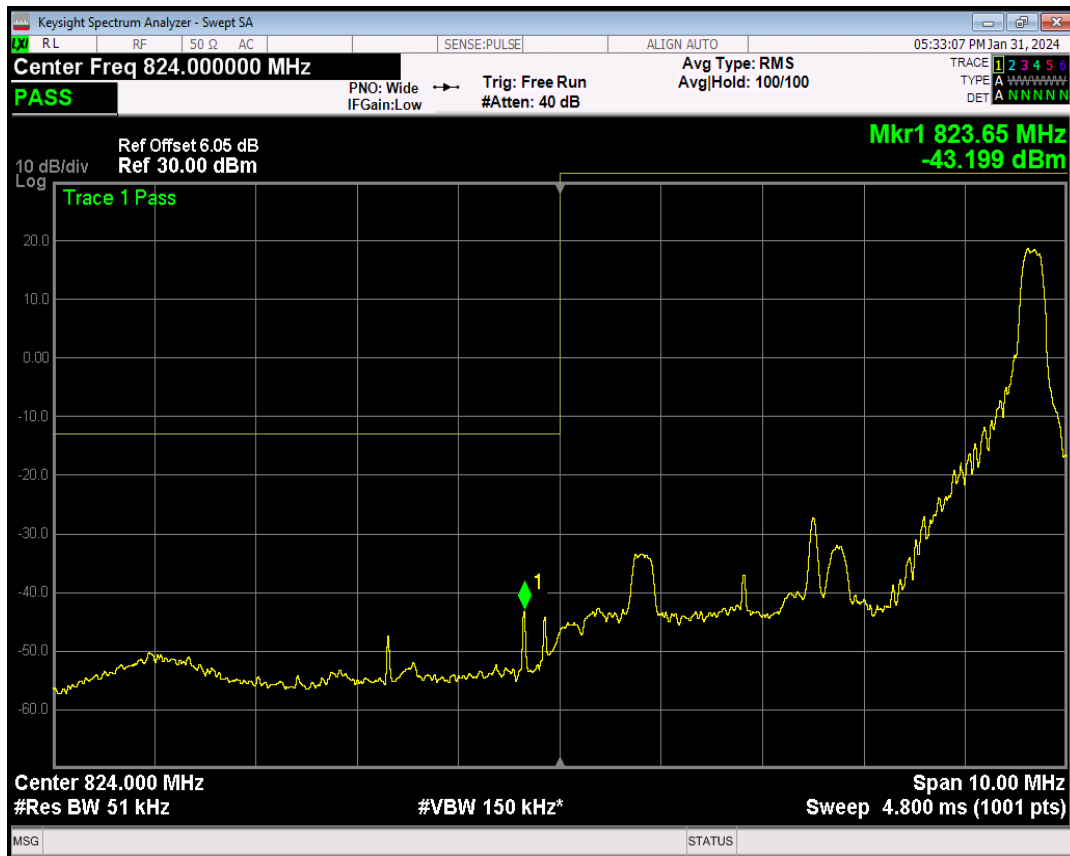
Band5 16QAM BW=5MHz Channel=20425 RB Size=25 Position=#0
