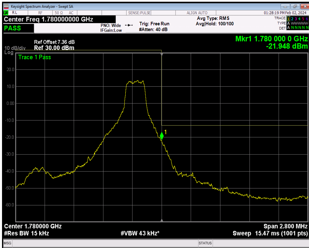
Band66 QPSK BW=1.4MHz Channel=132665 RB Size=6 Position=#0
