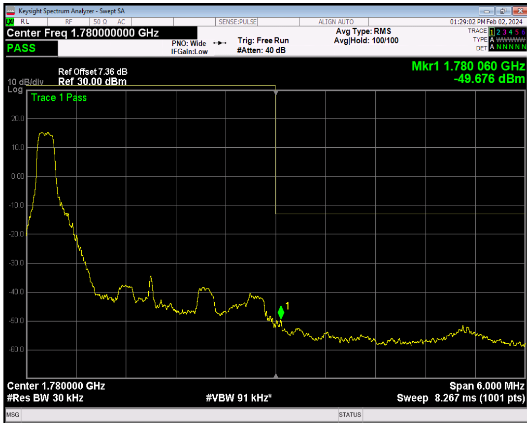
Band66 16QAM BW=3MHz Channel=132657 RB Size=1 Position=#Max
