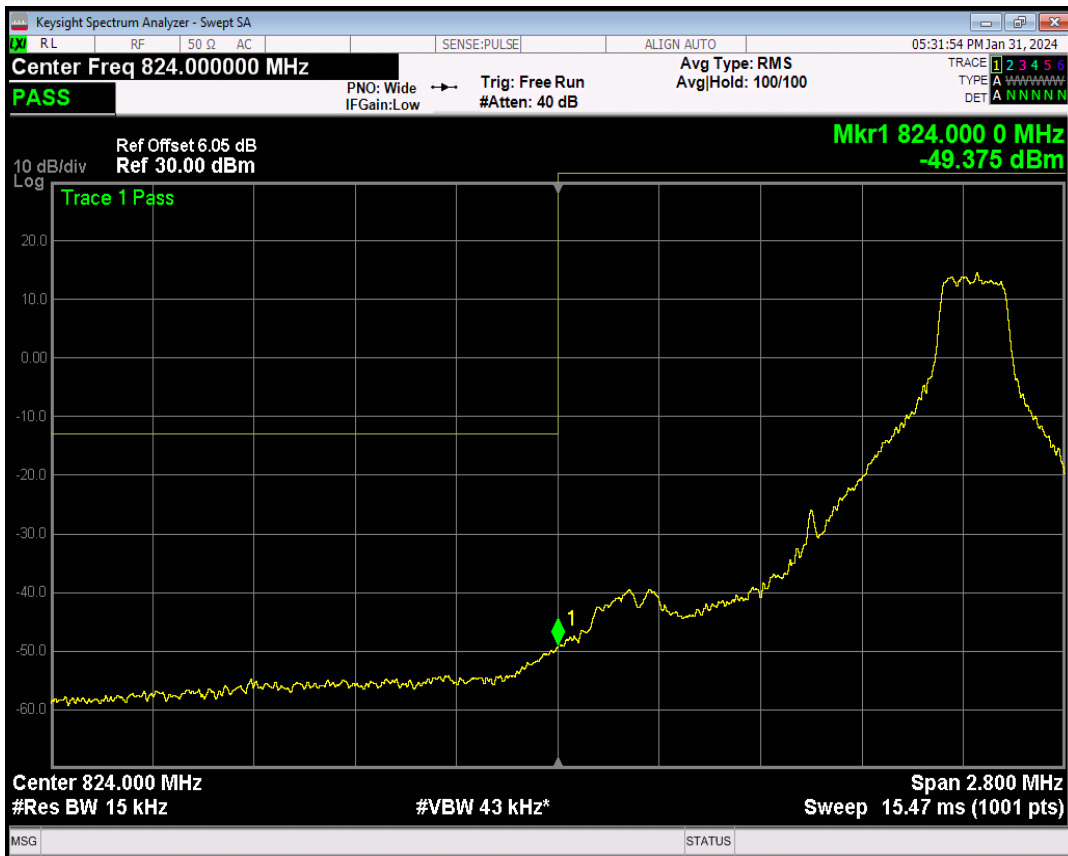
Band5 16QAM BW=1.4MHz Channel=20407 RB Size=6 Position=#0
