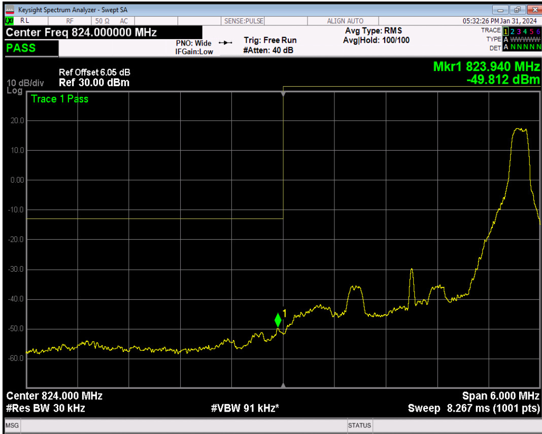
Band5 QPSK BW=3MHz Channel=20415 RB Size=15 Position=#0
