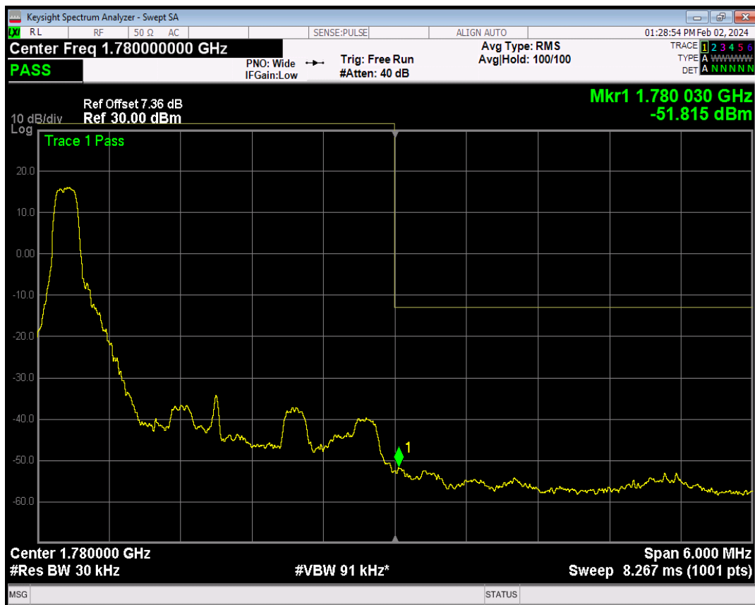
Band66 QPSK BW=3MHz Channel=132657 RB Size=1 Position=#Max
