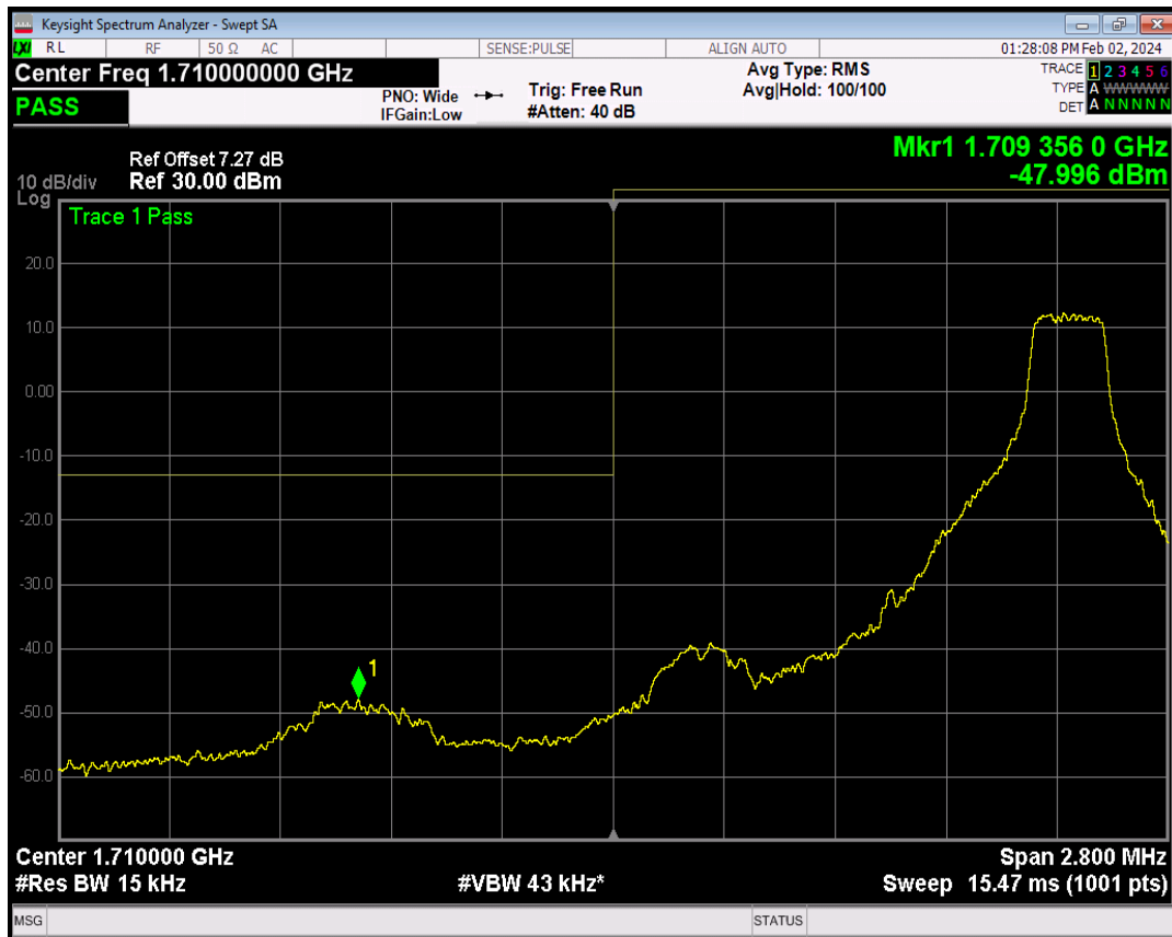
Band66 16QAM BW=1.4MHz Channel=131979 RB Size=6 Position=#0
