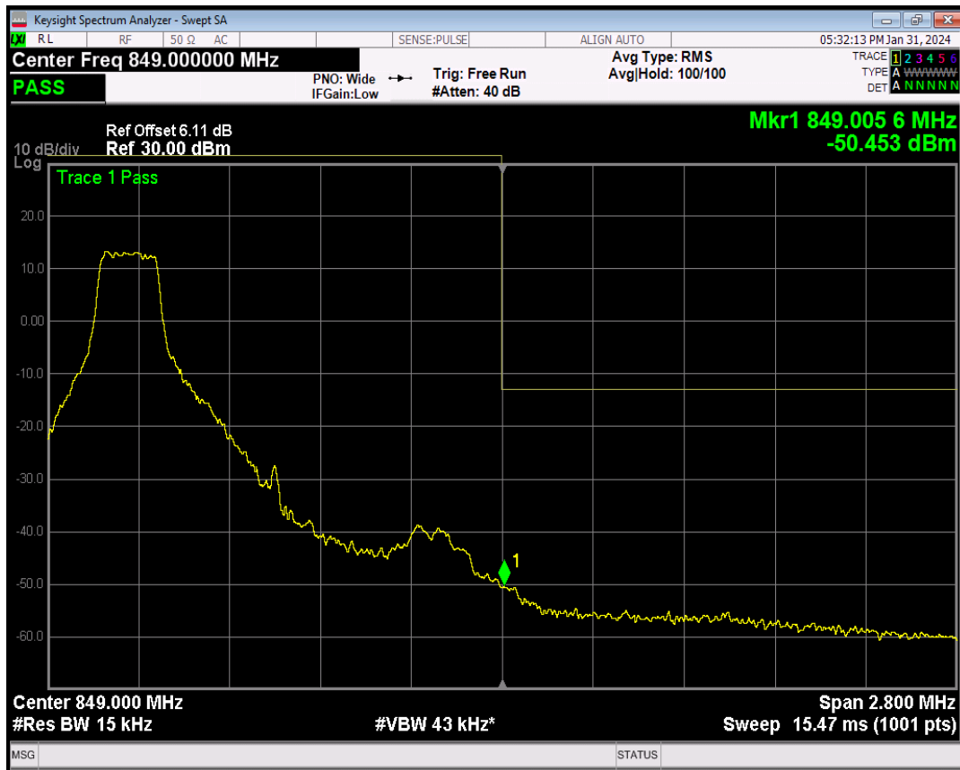
Band5 16QAM BW=1.4MHz Channel=20643 RB Size=1 Position=#Max
