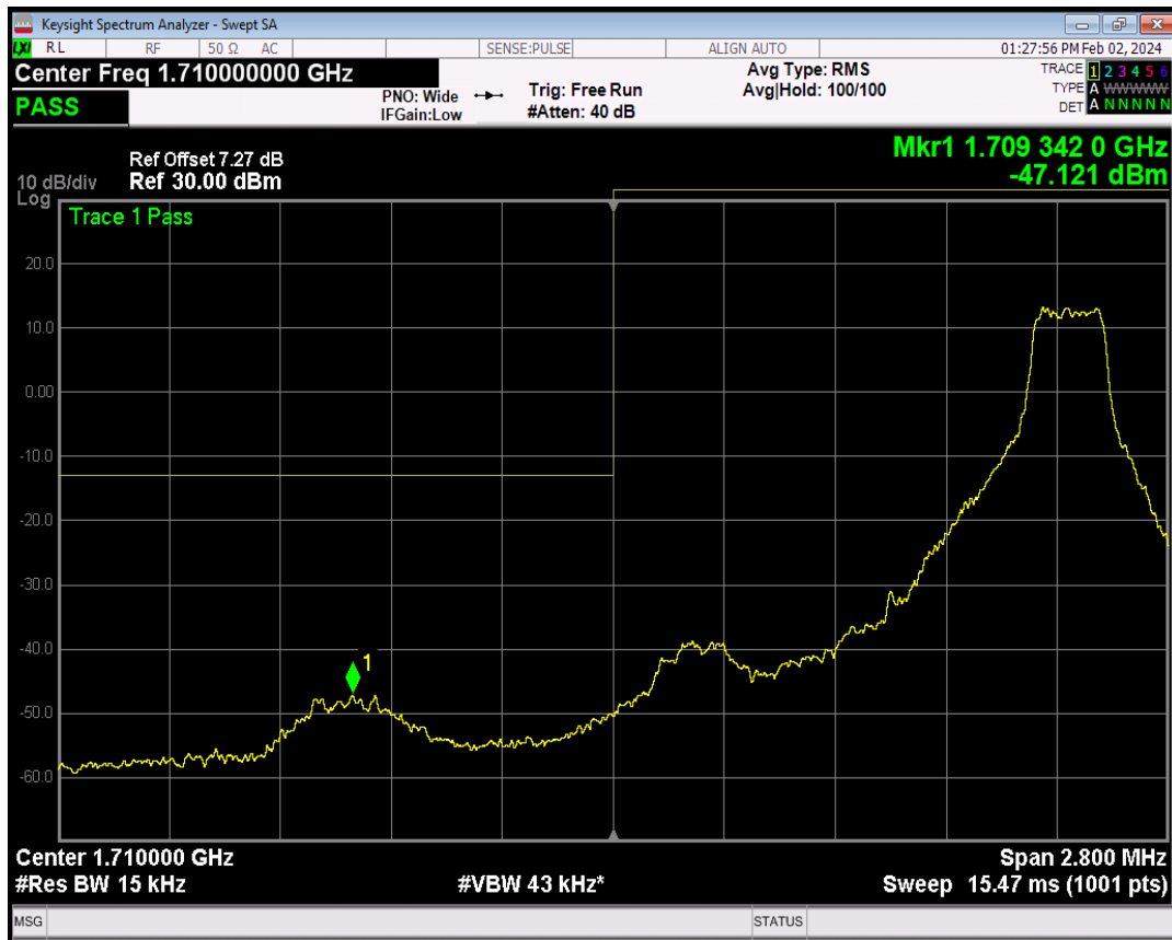
Band66 QPSK BW=1.4MHz Channel=131979 RB Size=6 Position=#0
