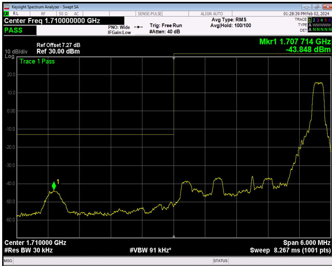
Band66 QPSK BW=3MHz Channel=131987 RB Size=15 Position=#0
