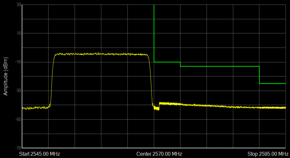
Band7 QPSK BW=20MHz Channel=21350 RB Size=100 Position=#0
