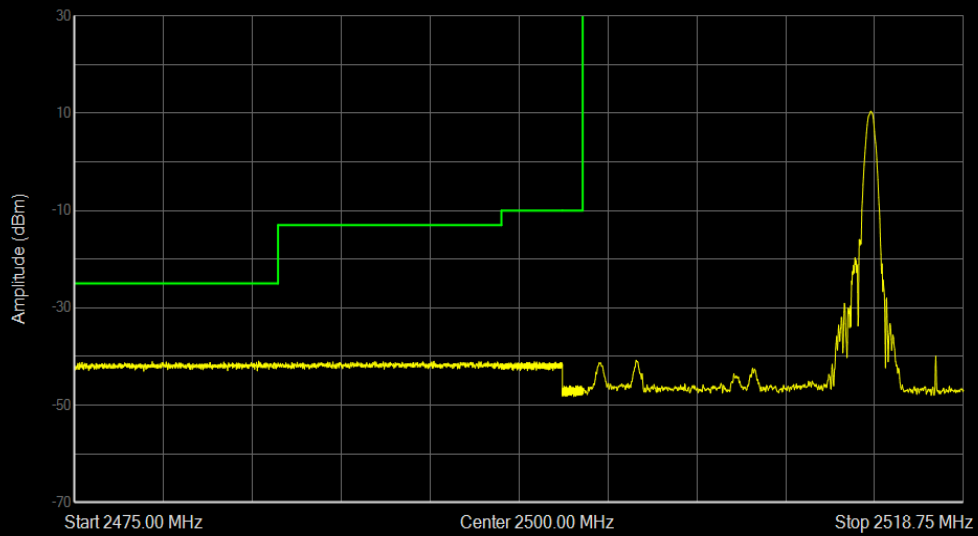
Band7 16QAM BW=15MHz Channel=20825 RB Size=1 Position=#Max
