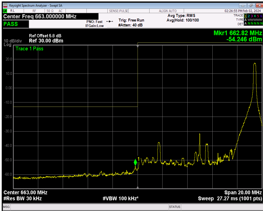
Band71 QPSK BW=10MHz Channel=133172 RB Size=50 Position=#0
