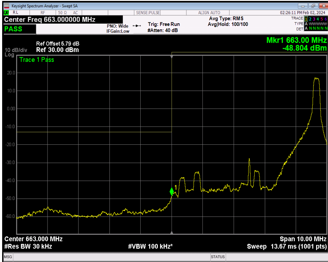
Band71 QPSK BW=5MHz Channel=133147 RB Size=25 Position=#0
