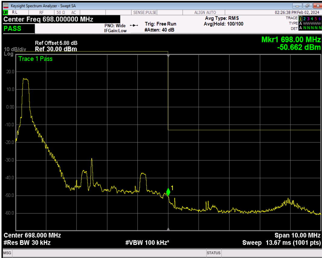
Band71 16QAM BW=5MHz Channel=133447 RB Size=1 Position=#Max
