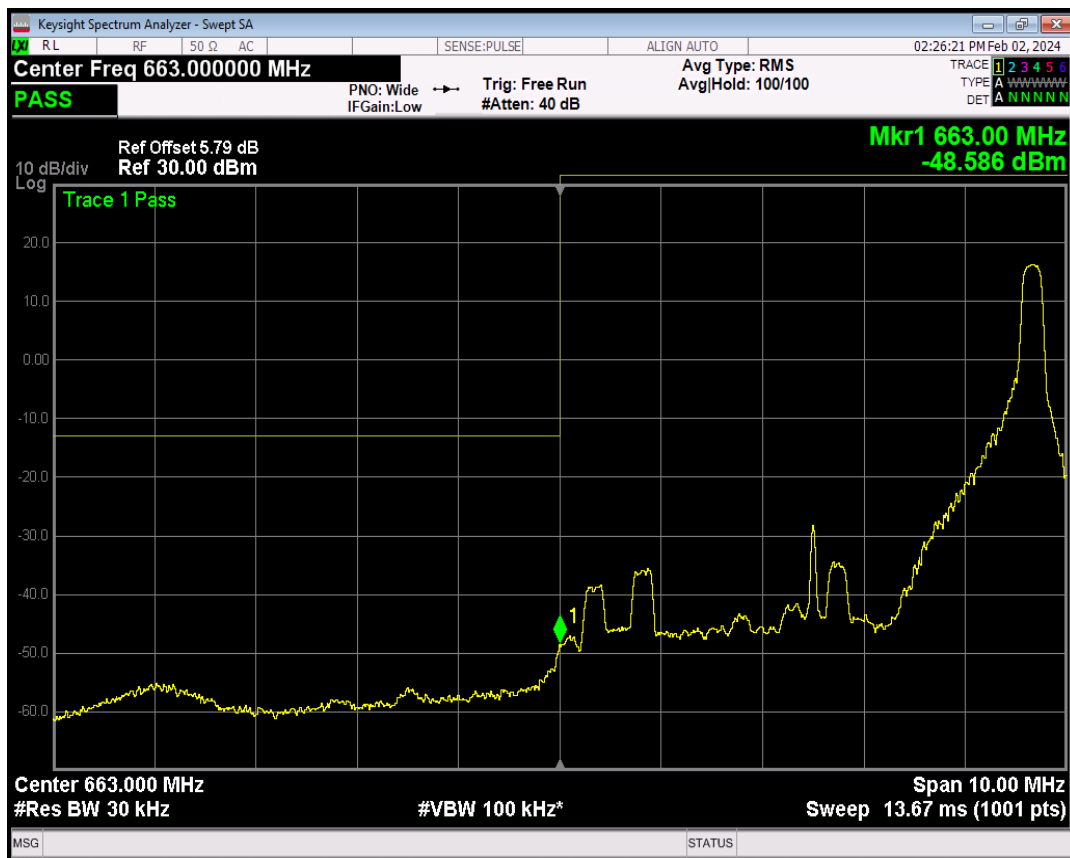
Band71 16QAM BW=5MHz Channel=133147 RB Size=25 Position=#0
