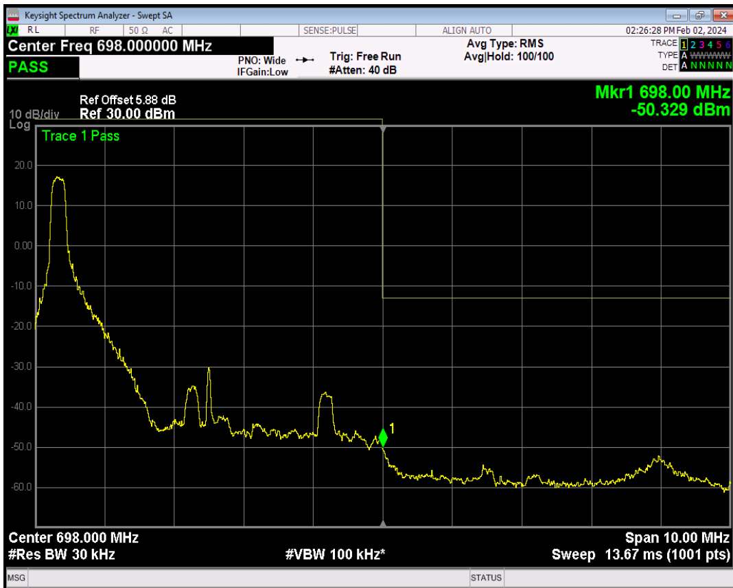
Band71 QPSK BW=5MHz Channel=133447 RB Size=1 Position=#Max
