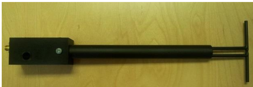
Figure 1 – MVG COMOSAR Validation Dipole
