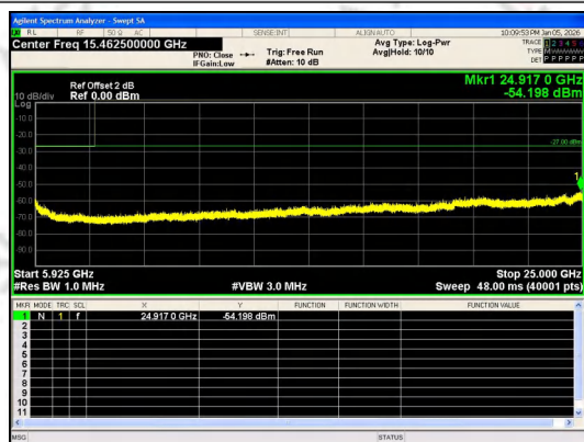
Spurious Emission:5925~25000.0 MHz IEEE 802.11ax_Channel 149_20MHz_Antenna 0 RU&Index SU
