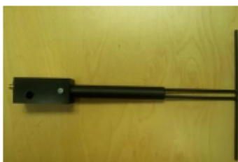
Figure 1 – MVG COMOSAR Validation Dipole
