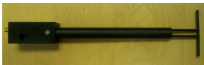
Figure 1 – MVG COMOSAR Validation Dipole
