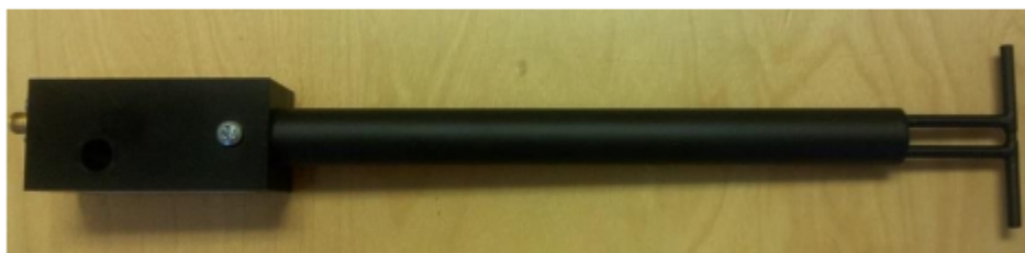
Figure 1 – MVG COMOSAR Validation Dipole
