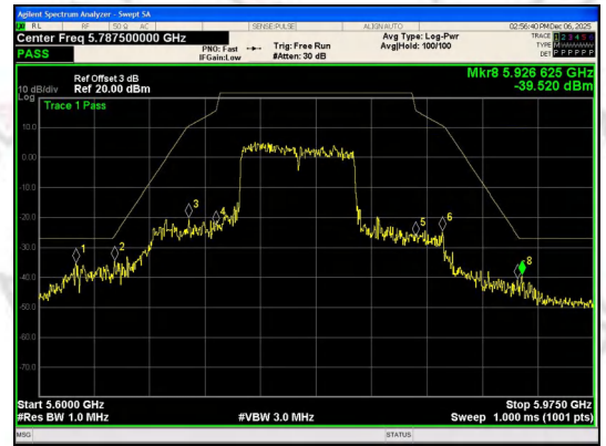
Out Of Band Emission IEEE 802.11ac_Channel 155_80MHz_Antenna 0
