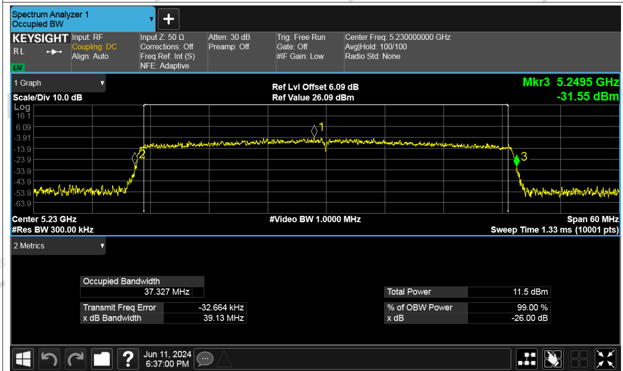
-26dB Bandwidth NVNT be40 5230MHz Ant2
