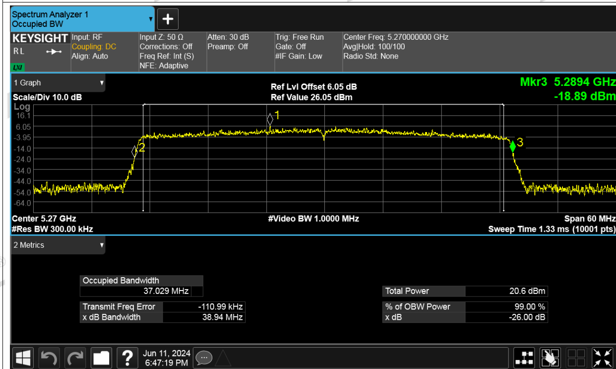
-26dB Bandwidth NVNT be40 5270MHz Ant3
