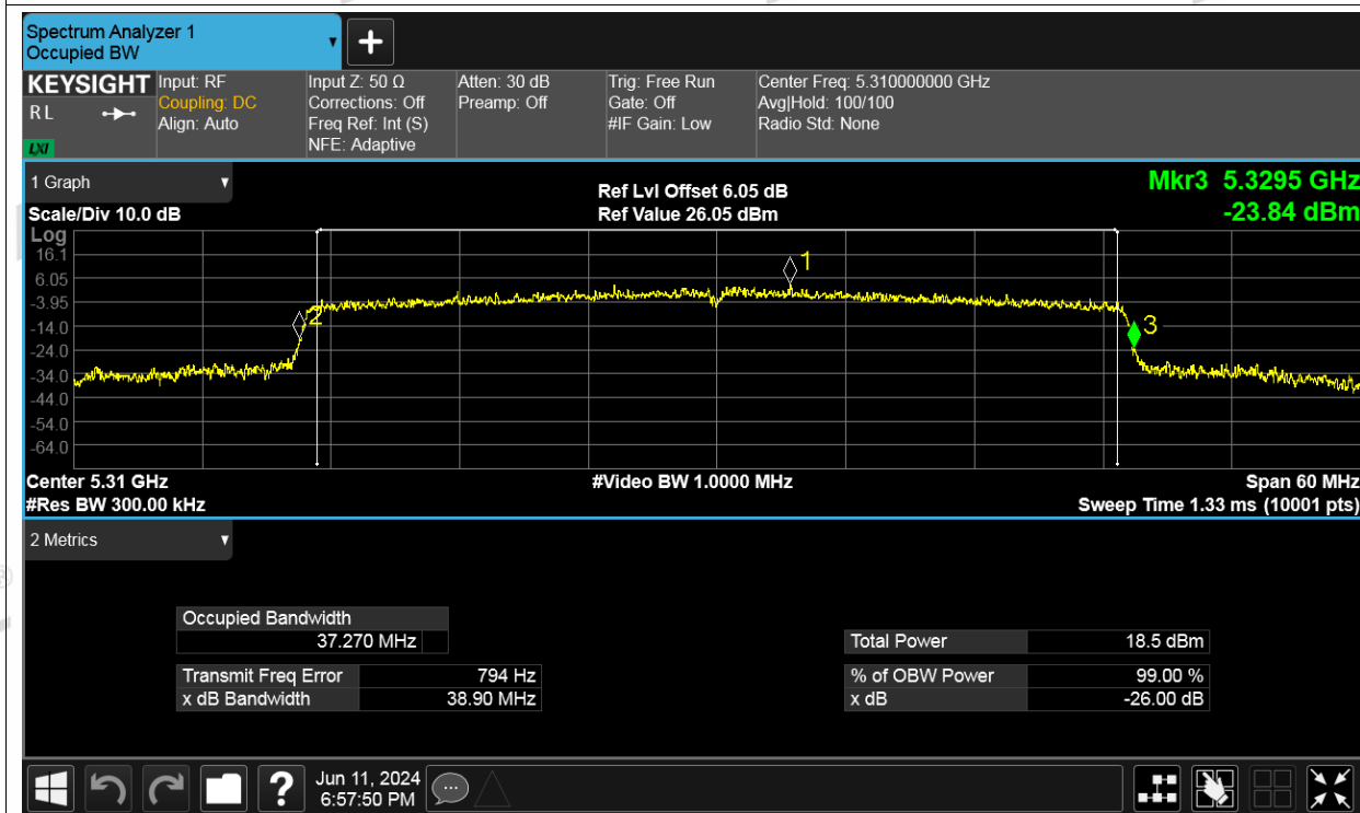
-26dB Bandwidth NVNT be40 5310MHz Ant2
