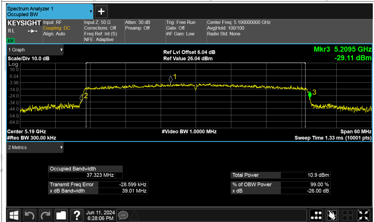
-26dB Bandwidth NVNT be40 5190MHz Ant3
