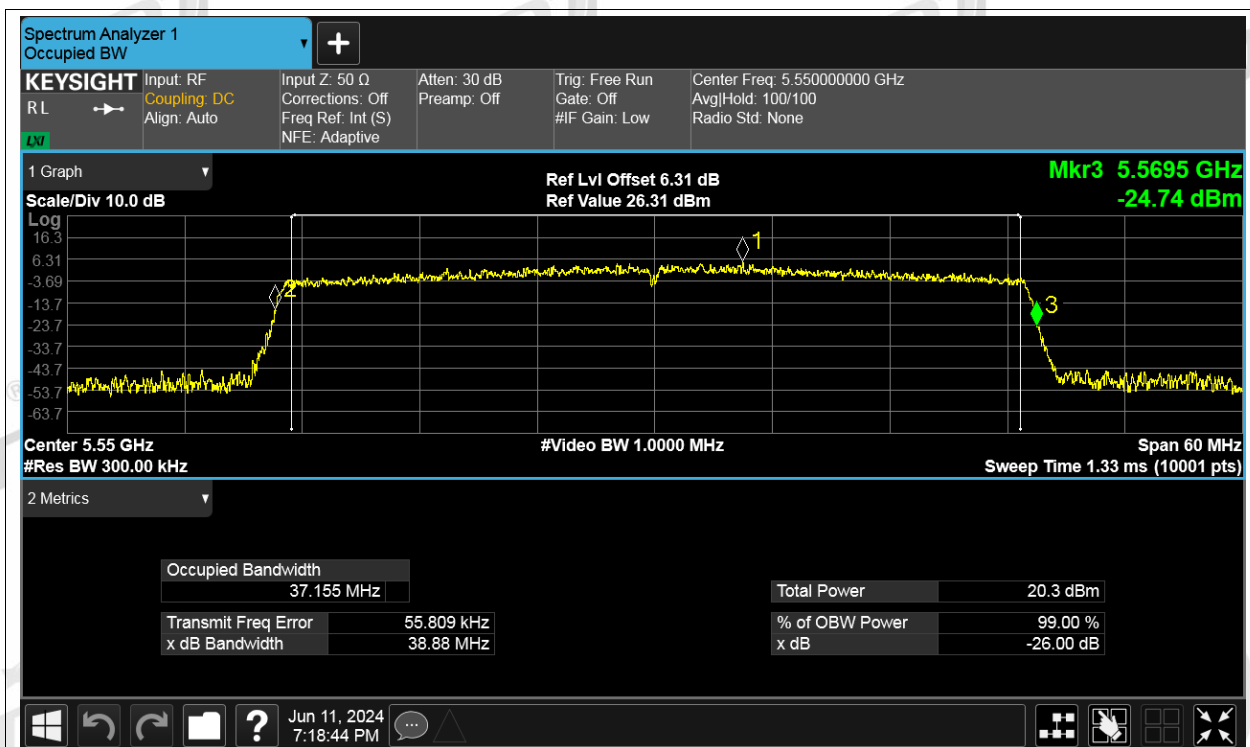
-26dB Bandwidth NVNT be40 5550MHz Ant3
