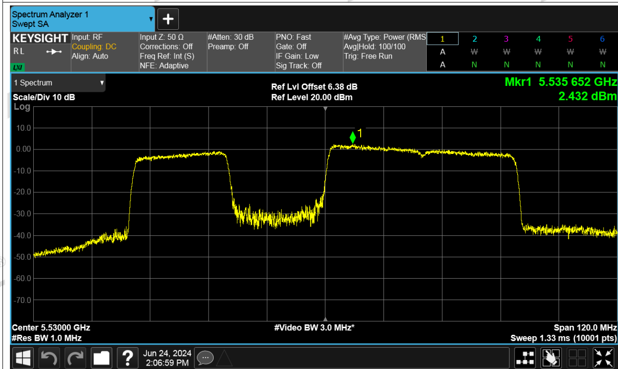
PSD NVNT be80 484+242-tone in a non-OFDMA MRU2 5610MHz Ant1
