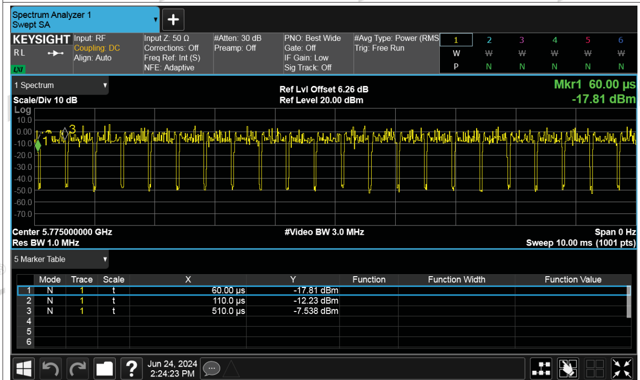
Duty Cycle NVNT be80 484+242-tone in a non-OFDMA MRU1 5210MHz Sum
