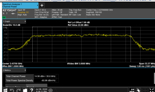
Conducted Output Power IEEE 802.11n 40 Channel 6 Antenna 0
