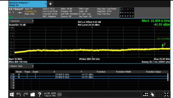
30.0 MHz - 25000.0 MHz IEEE 802.11g Channel 11 20MHz Antenna 0
