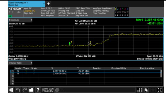
Out Of Band Emission IEEE 802.11n Channel 1 20MHz Antenna 0
