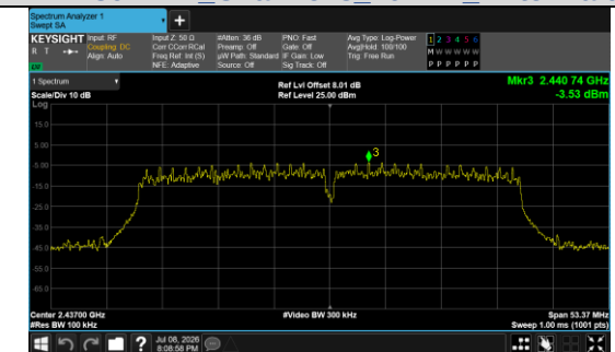
In-Band Reference Level IEEE 802.11n Channel 6 40MHz Antenna 0
