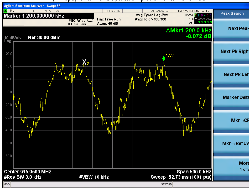
(1Mbps) Channel Separation plot on channel 102-103
