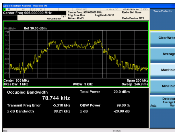
20dB Bandwidth plot on channel 01 (1Mbps)
