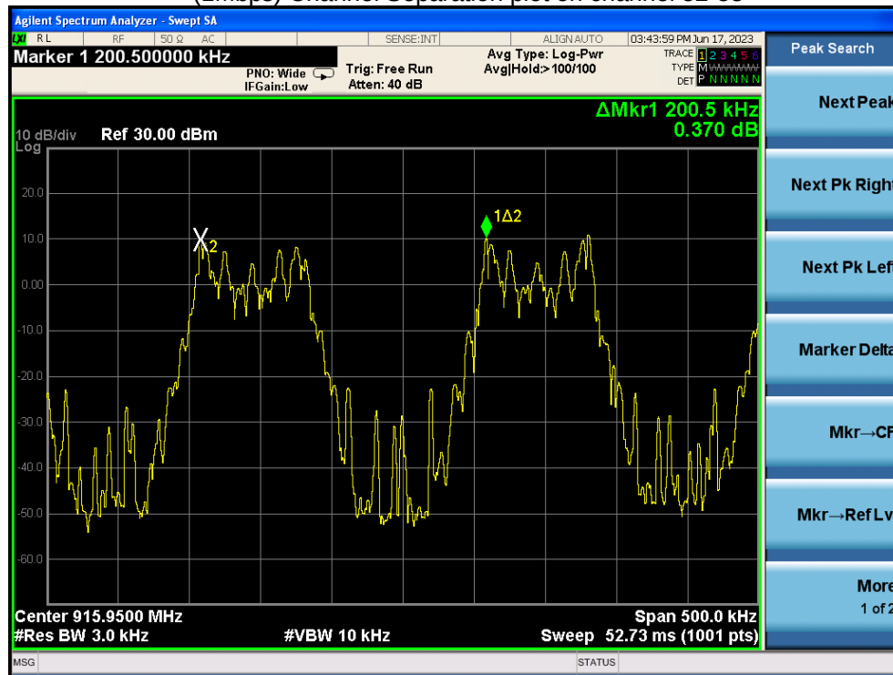
(1Mbps) Channel Separation plot on channel 102-103
