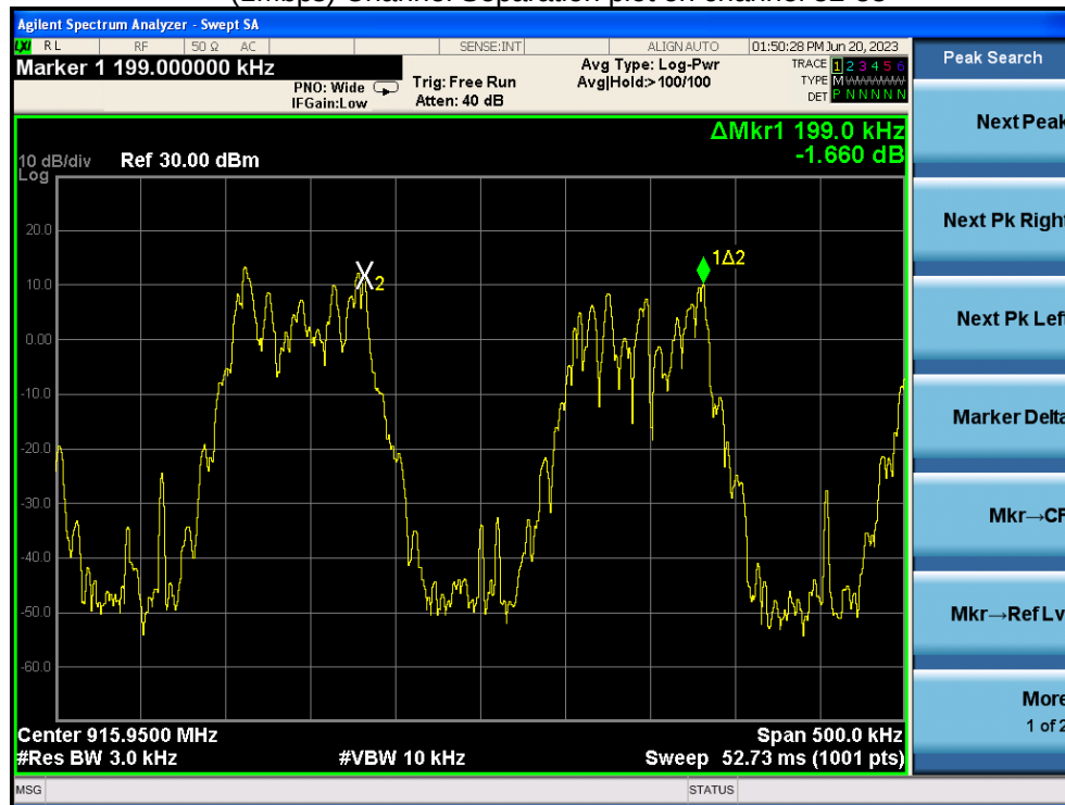
(1Mbps) Channel Separation plot on channel 102-103
