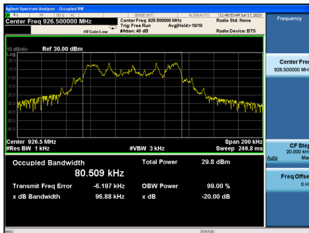
20dB Bandwidth plot on channel 103 (1Mbps)
