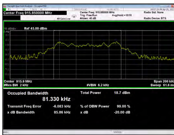
20dB Bandwidth plot on channel 52 (1Mbps)
