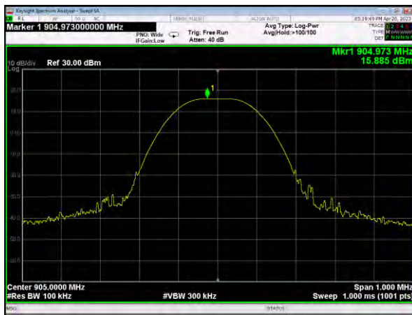
Peak output Power plot on channel 103 (1Mbps)
