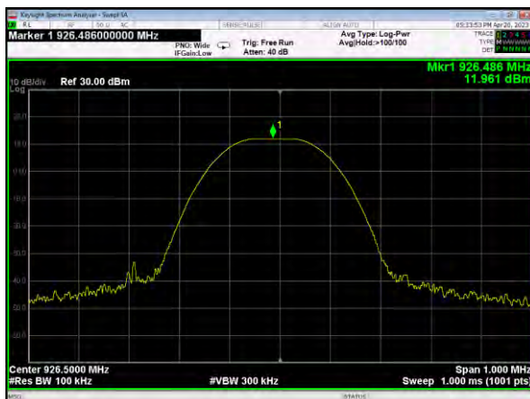
Peak output Power plot on channel 103 (1Mbps)
