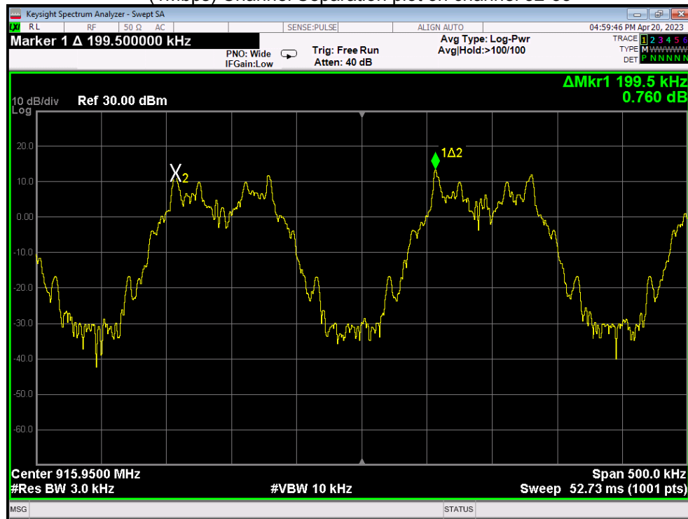
(1Mbps) Channel Separation plot on channel 102-103
