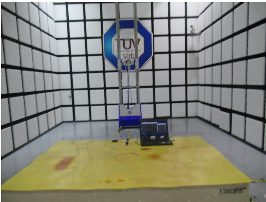
Radiated Emission Test below 1GHz
