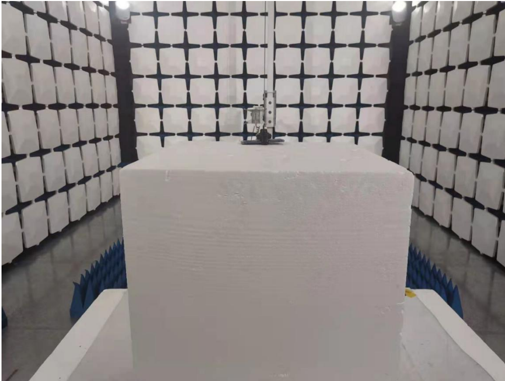
Above 1GHz for radiated emission test setup
