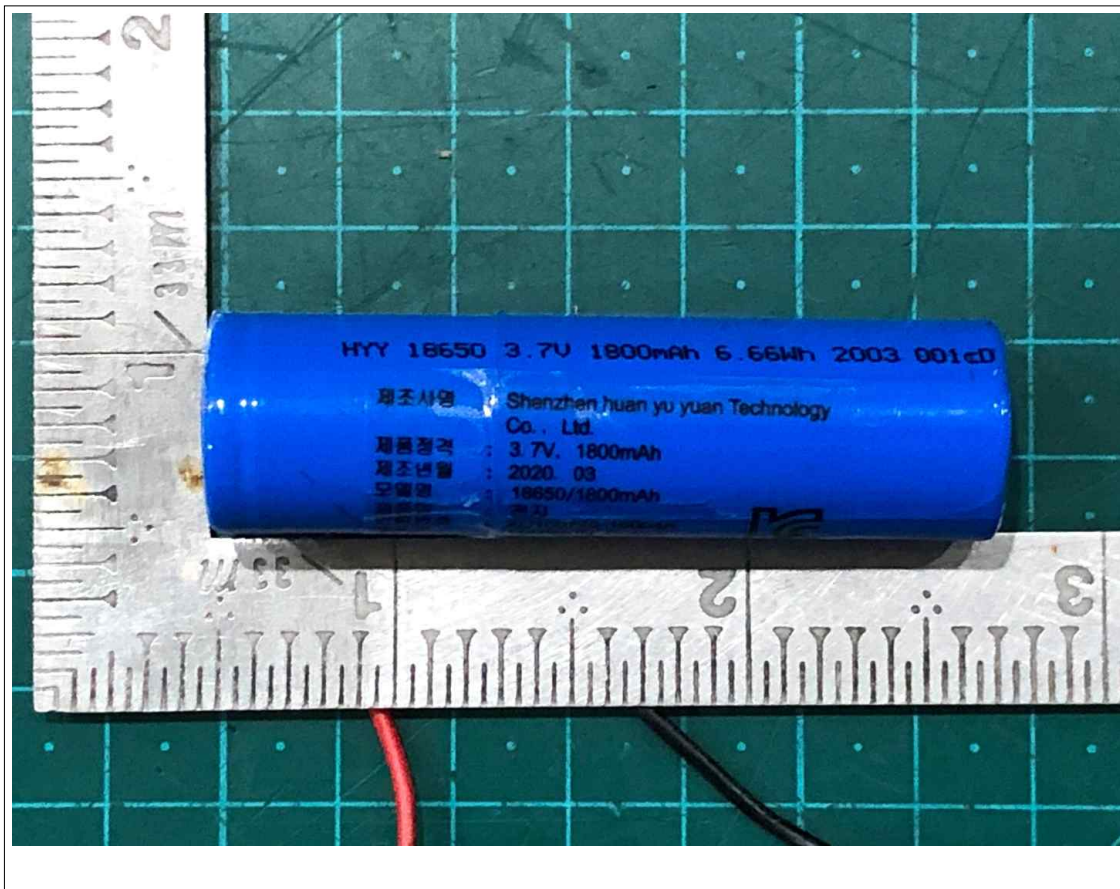
View of Battery (Top)
