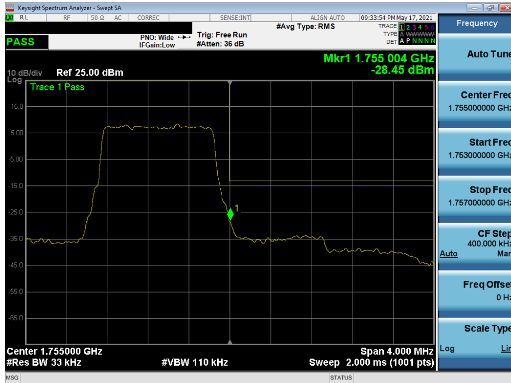
Plot 7-88. Upper Band Edge Plot (LTE Band 4 – 1.4MHz QPSK – Full RB)
