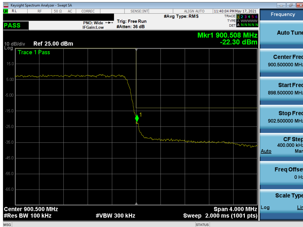
Plot 7-91. Upper Band Edge Plot (LTE BAND 8 - 3MHz QPSK – Full RB)
