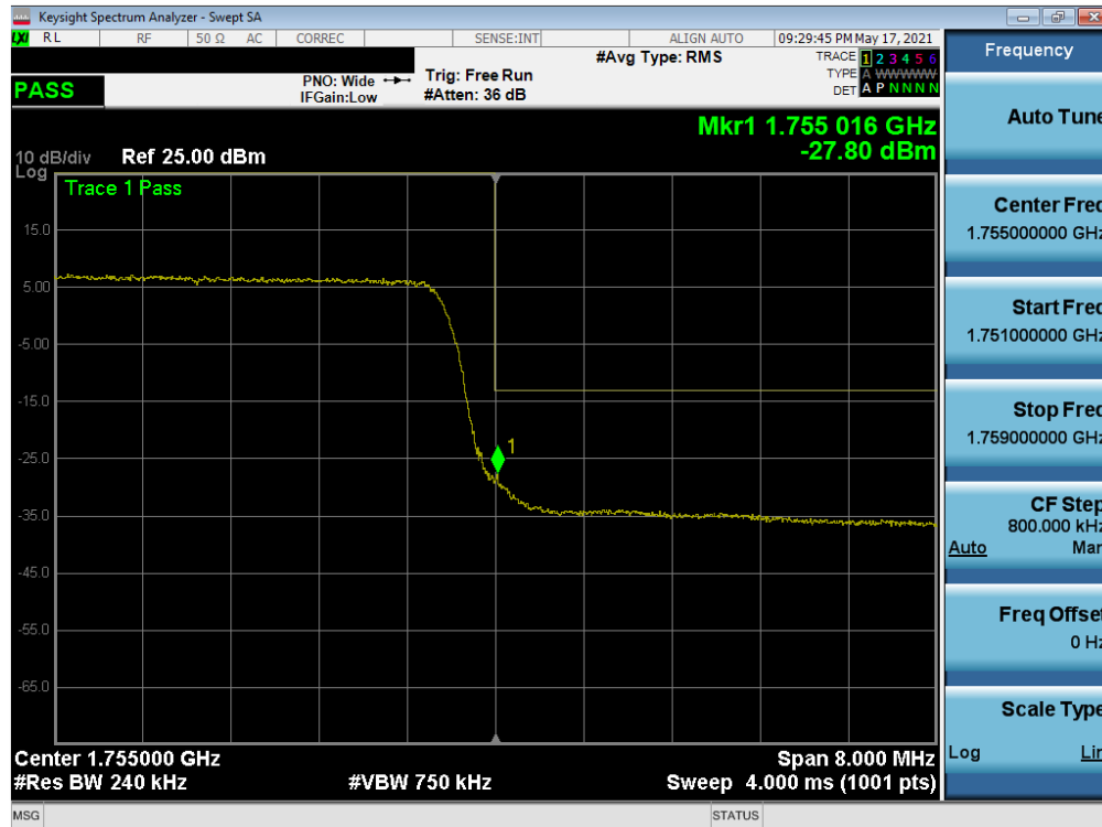
Plot 7-76. Upper Band Edge Plot (LTE Band 4 - 10MHz QPSK – Full RB)
