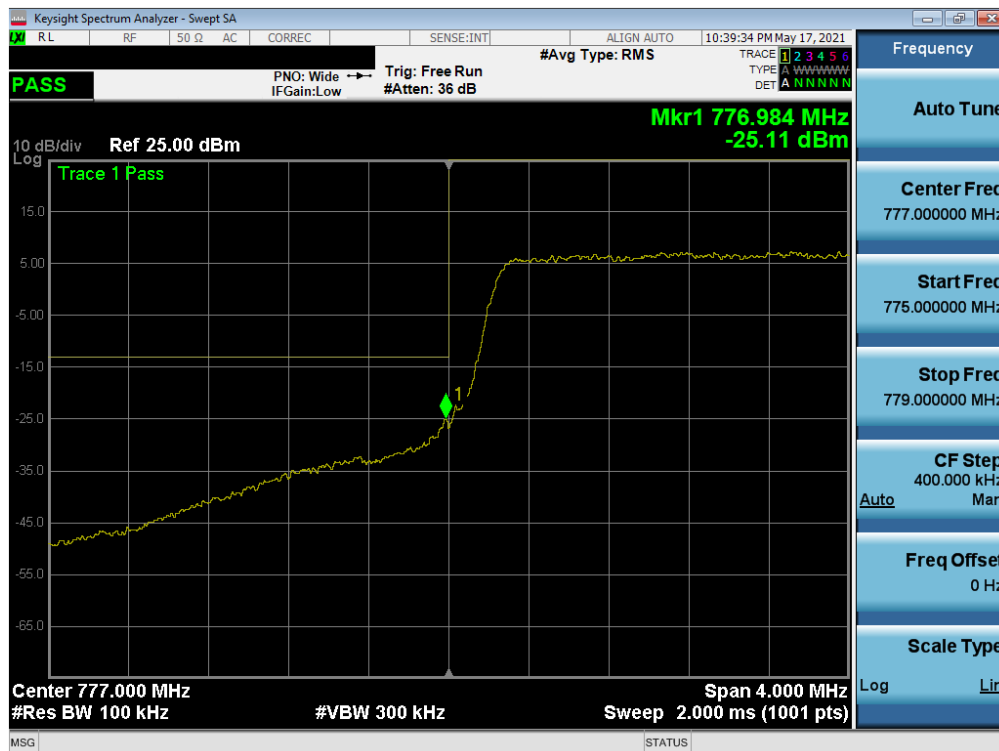
Plot 7-106. Lower Band Edge Plot (LTE Band 13 - 5MHz QPSK - Full RB)
