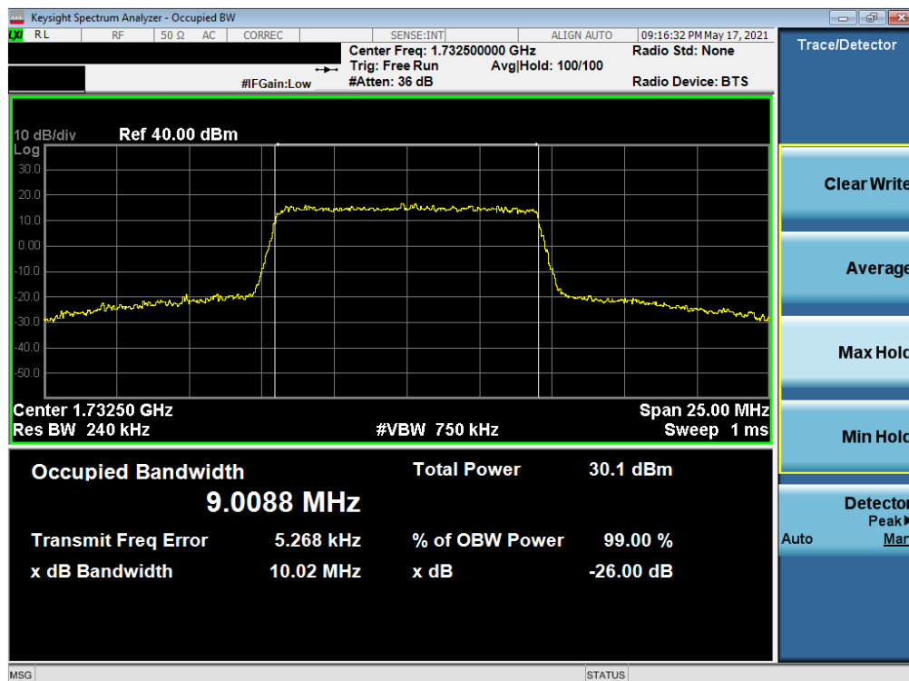
Plot 7-6. Occupied Bandwidth Plot (LTE Band 4 - 10MHz 16-QAM - Full RB)
