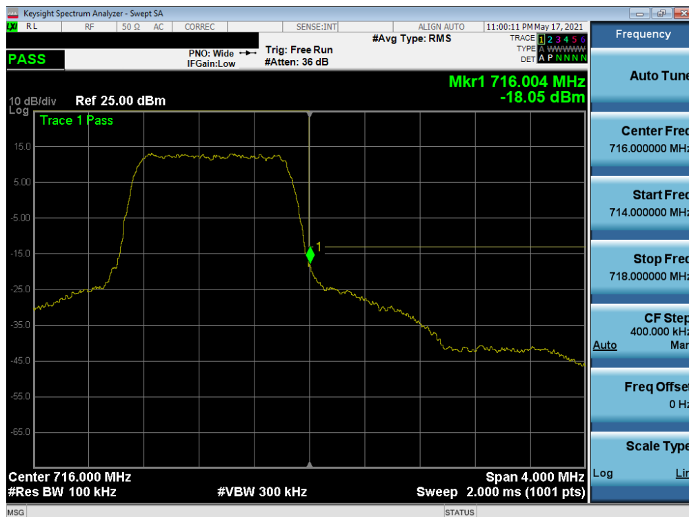
Plot 7-101. Upper Band Edge Plot (LTE Band 12 - 1.4MHz QPSK - Full RB)
