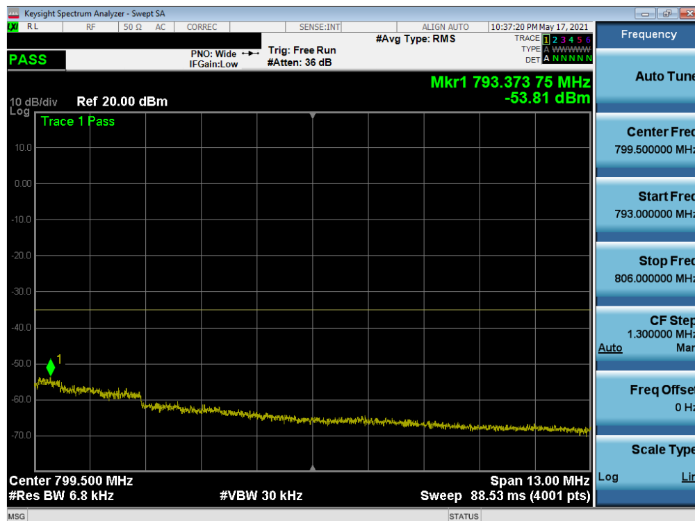
Plot 7-105. Upper Emission Mask Plot (LTE Band 13 - 10MHz QPSK – Full RB)
