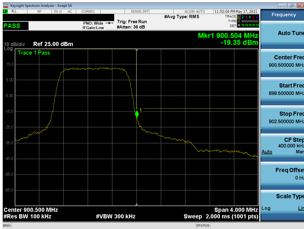
Plot 7-93. Upper Band Edge Plot (LTE BAND 8 – 1.4MHz QPSK – Full RB)
