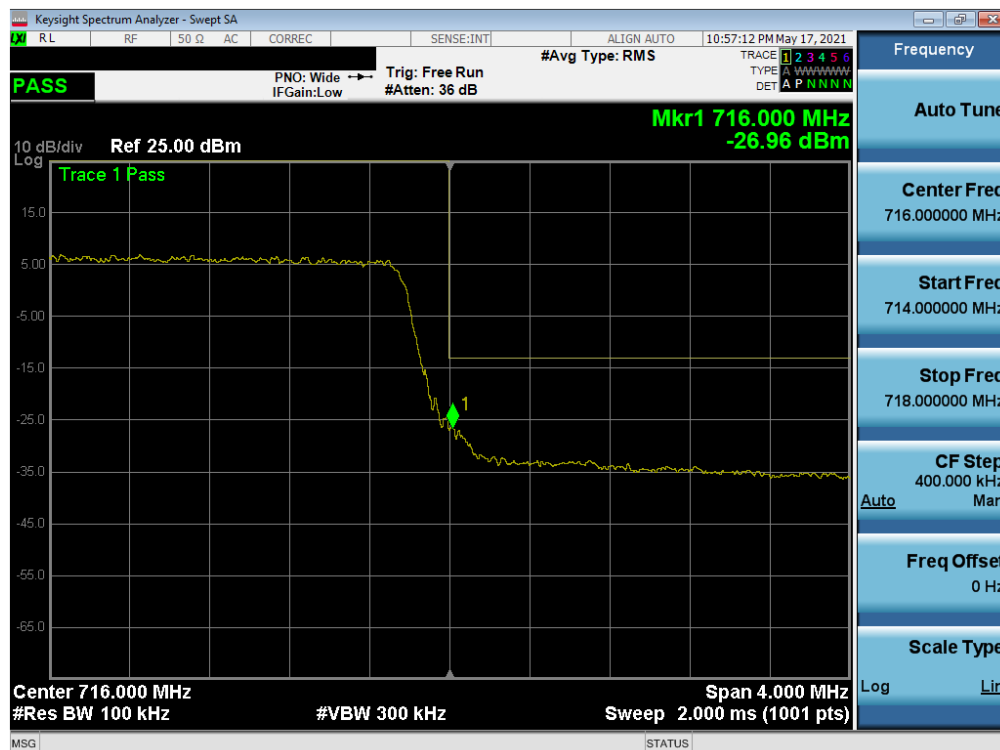
Plot 7-97. Upper Band Edge Plot (LTE Band 12 - 5MHz QPSK - Full RB)
