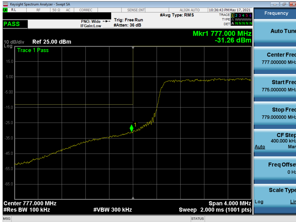
Plot 7-102. Lower Band Edge Plot (LTE Band 13 - 10MHz QPSK – Full RB)
