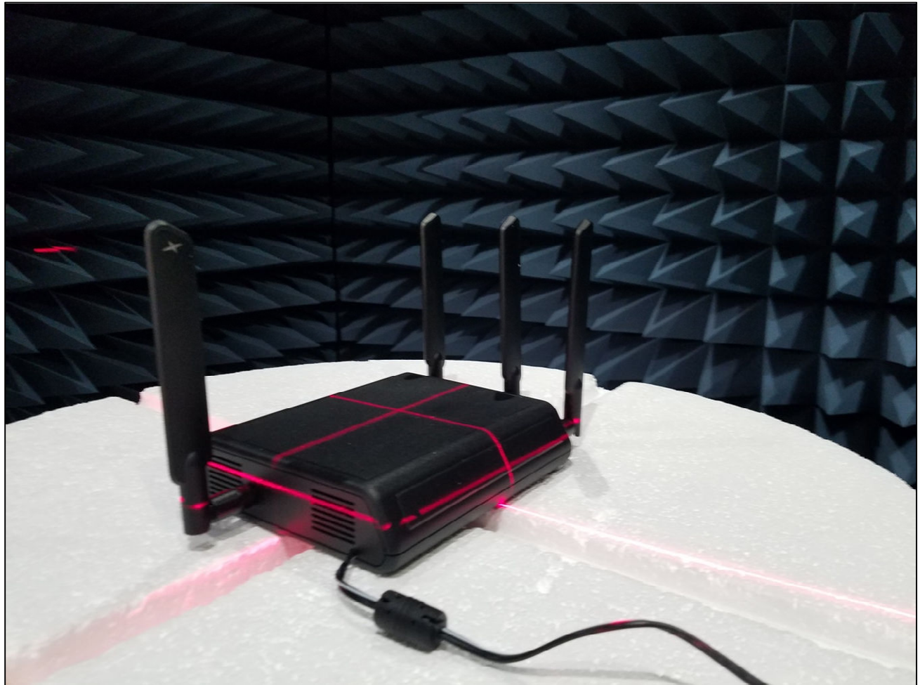
OTA EIRP Test Setup View 1
