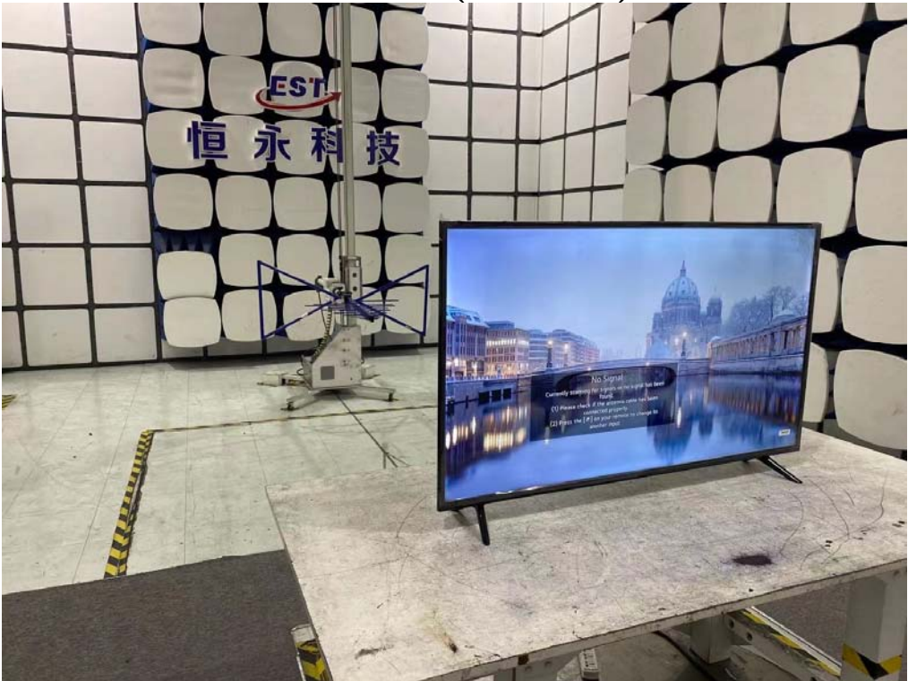
Radiated Test (Below 1GHz)
