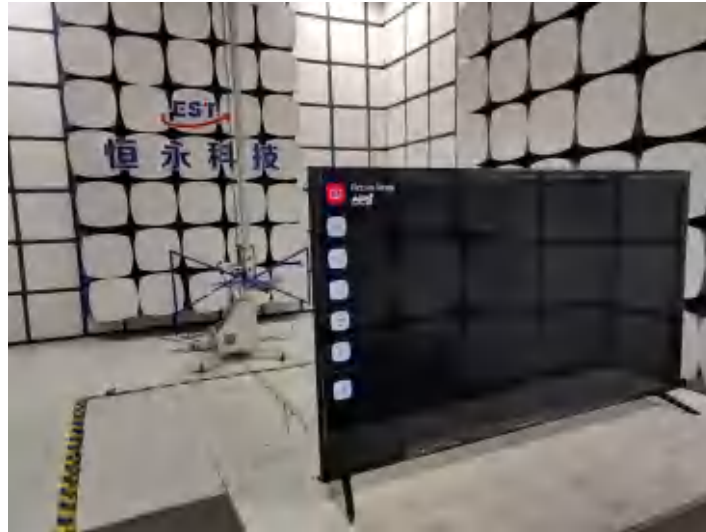
Radiated Test (Below 1GHz)
