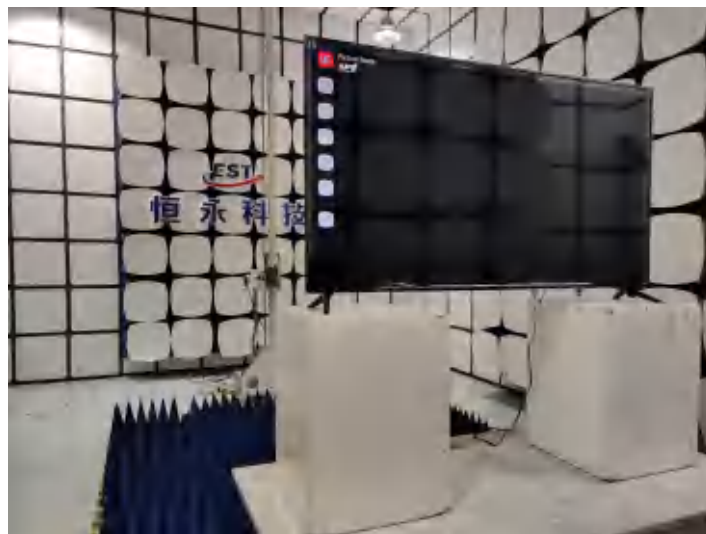
Radiated Test (Above 1GHz)
