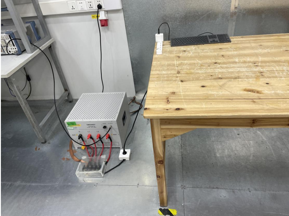
Photo of Conducted Emission Measurement
