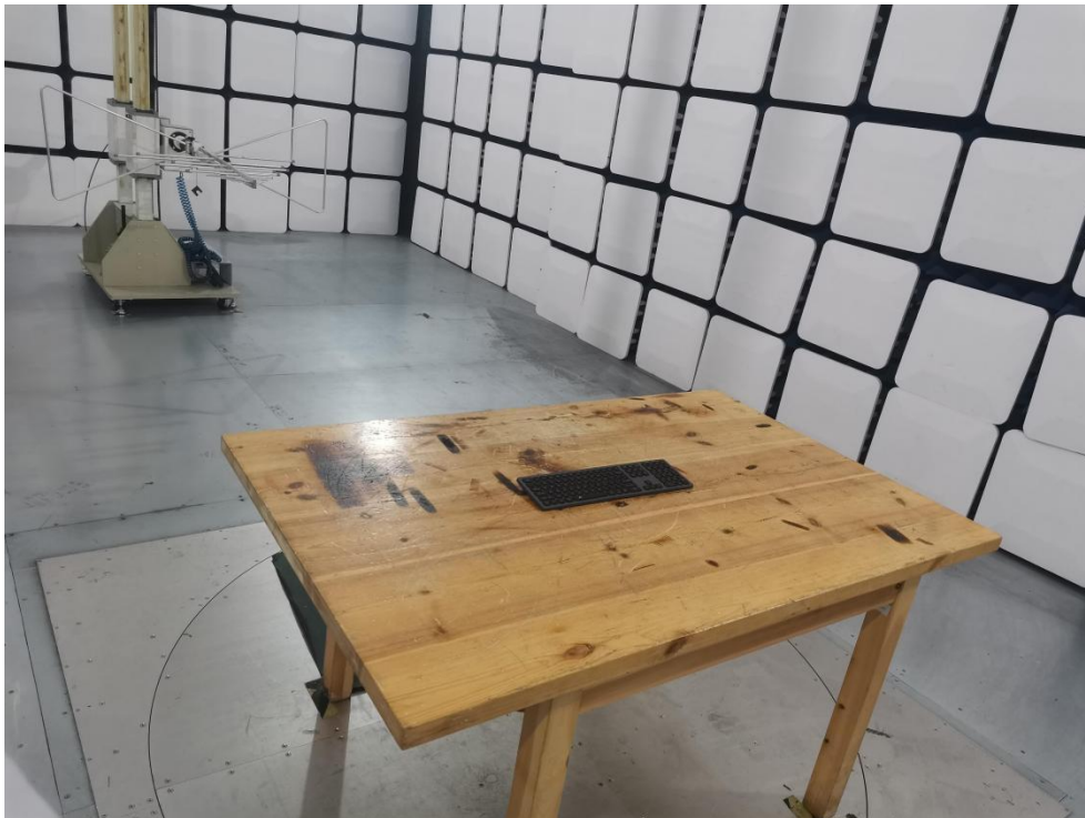
Photo of Radiation Emission Test
