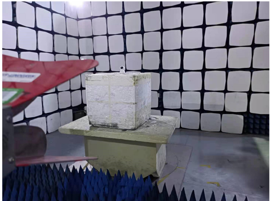
Radiation Emission Test Setup (1GHz to 18GHz)
