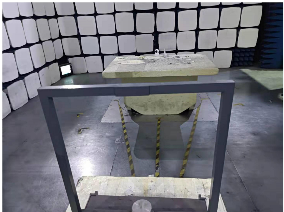
Radiation Emission Test Setup (Below 30MHz)
