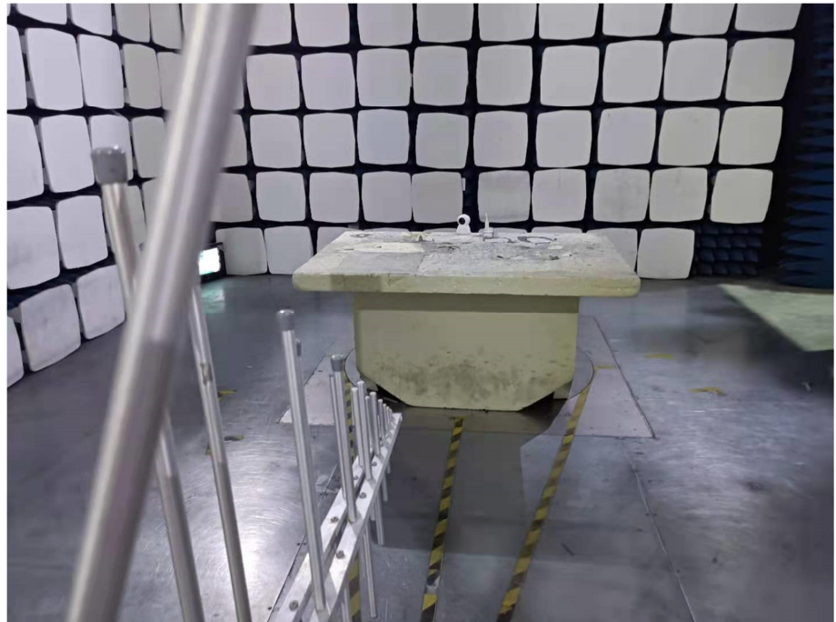
Radiation Emission Test Setup (30MHz to 1GHz)
