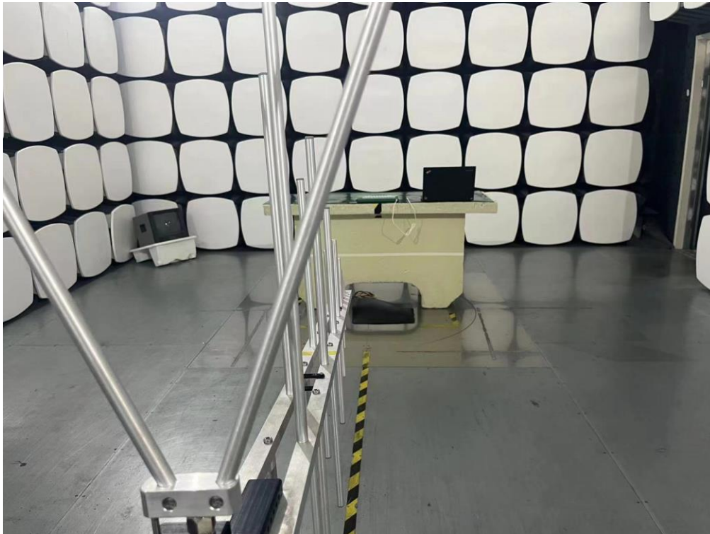
Radiated Emissions Test Photos 30 MHz to 1000 MHz
