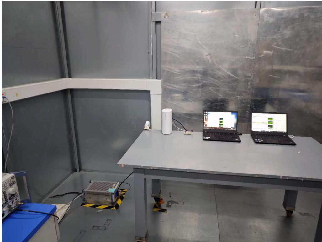
Photograph 3: Set-up photo for AC Conducted Emission
