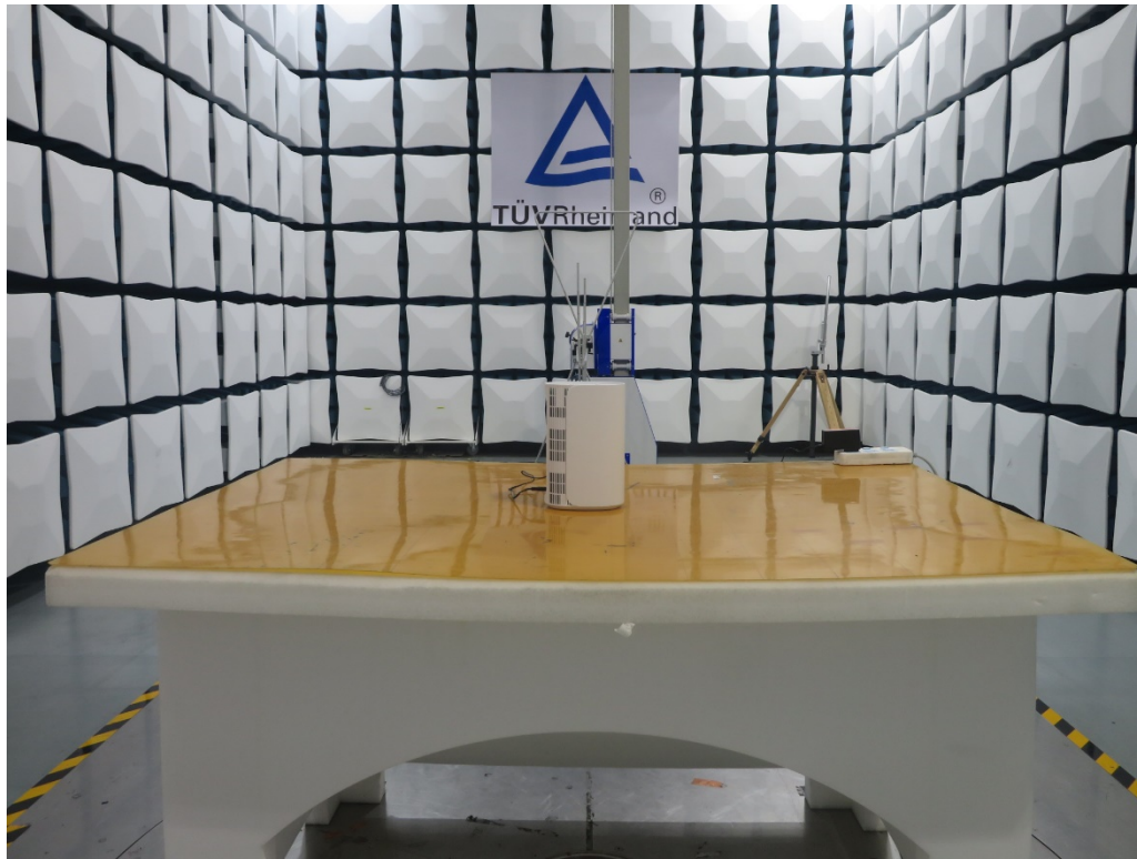
Photograph 1: Set-up photo for Radiated Spurious Emission, 30MHz - 1GHz
