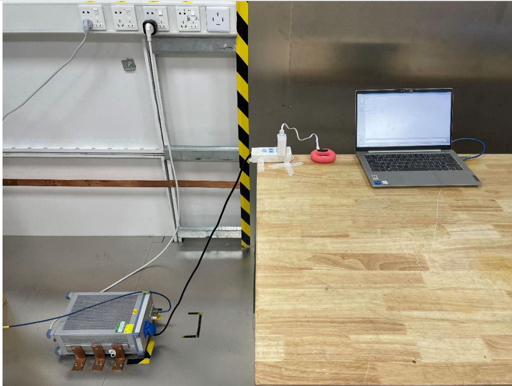
AC Power Line Conducted Emission
