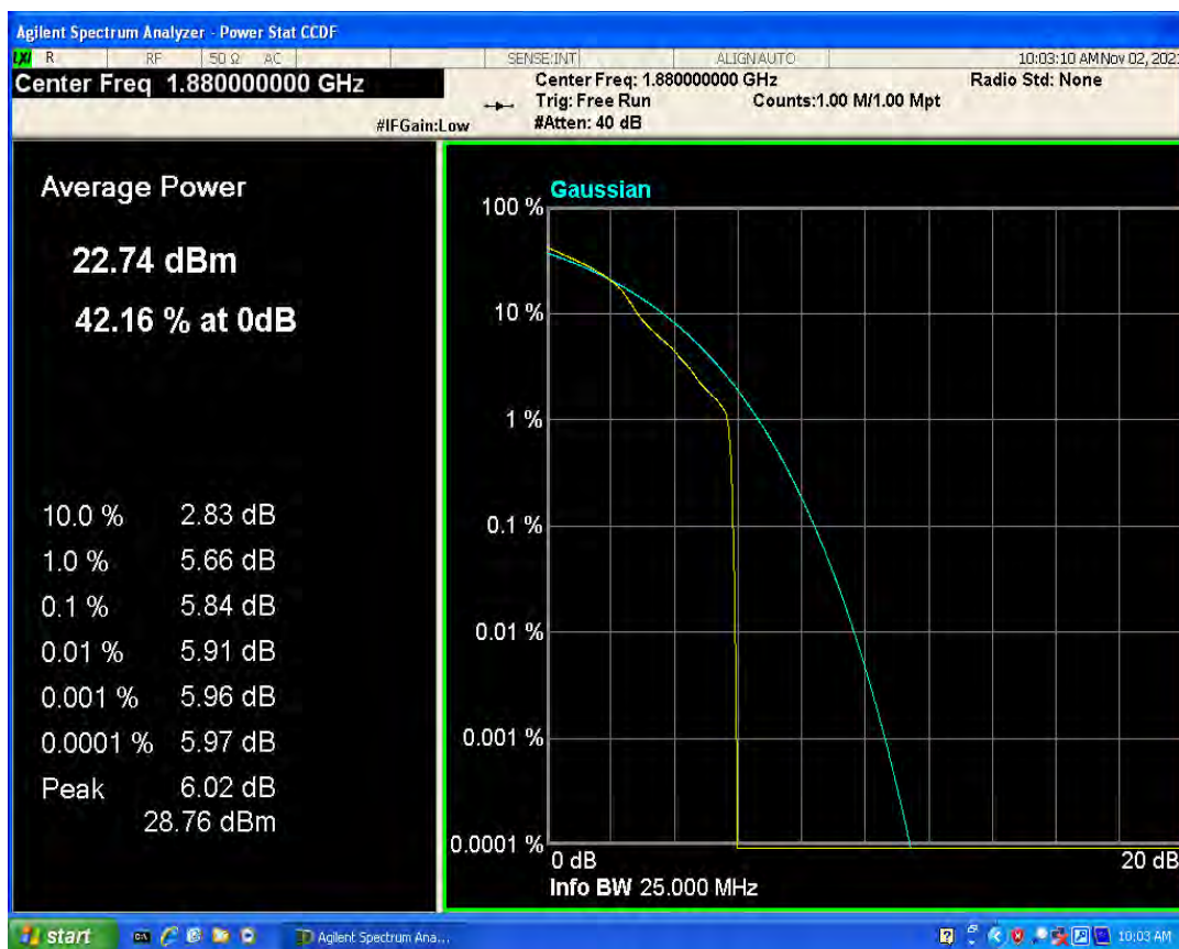
Band2 QPSK BW=15MHz Channel=18900 RB Size=1 Position=#0
