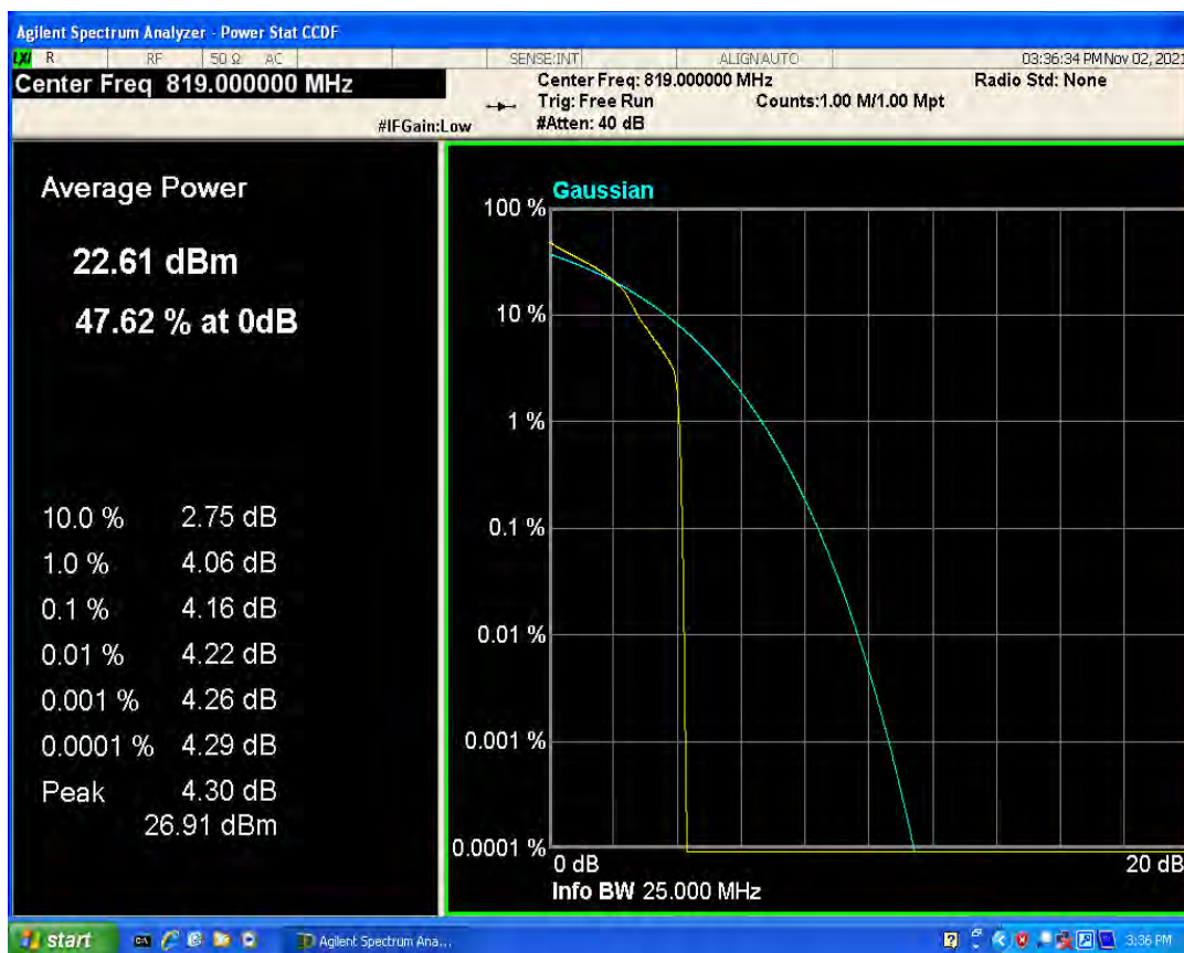
Band26a QPSK BW=5MHz Channel=26740 RB Size=1 Position=#0
