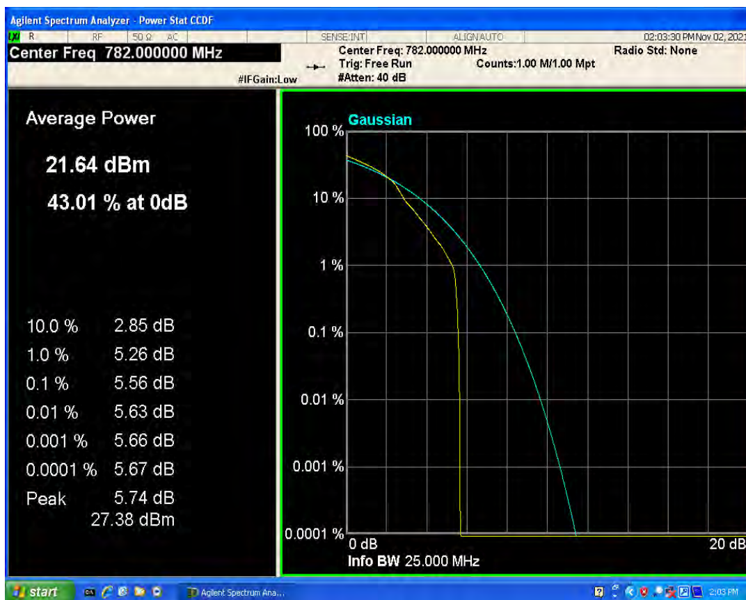
Band13 QAM16 BW=10MHz Channel=23230 RB Size=1 Position=#0
