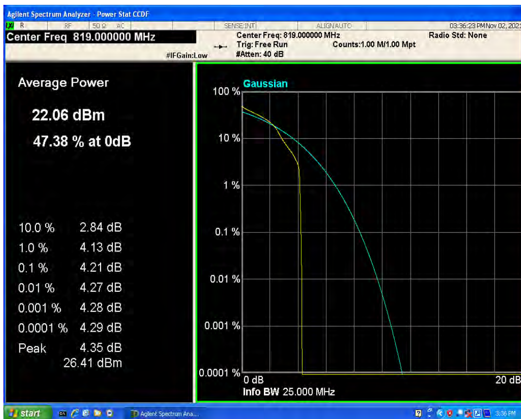
Band26a QPSK BW=3MHz Channel=26740 RB Size=1 Position=#0
