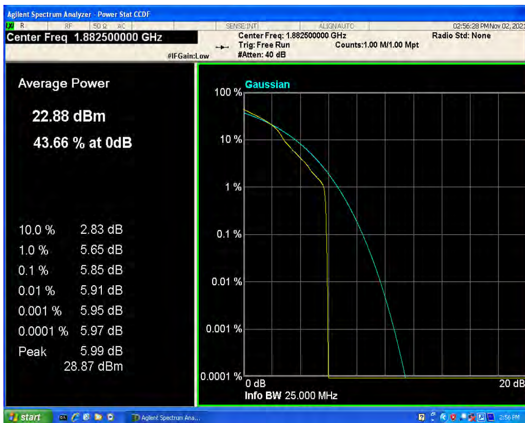
Band25 QPSK BW=15MHz Channel=26365 RB Size=1 Position=#0
