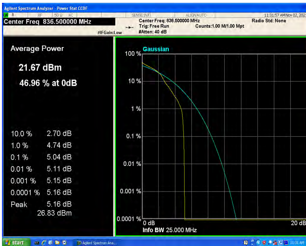
Band5 QPSK BW=10MHz Channel=20525 RB Size=1 Position=#0
