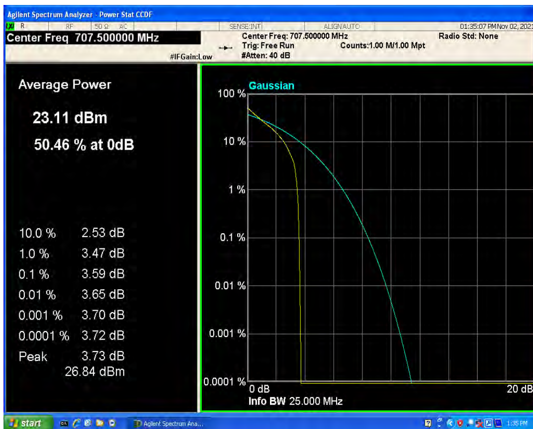
Band12 QAM16 BW=1.4MHz Channel=23095 RB Size=1 Position=#0
