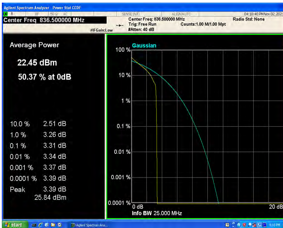
Band26b QAM16 BW=15MHz Channel=26915 RB Size=1 Position=#0
