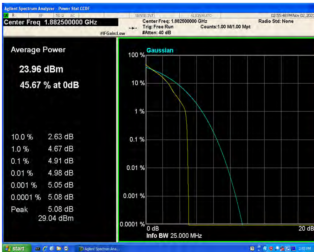
Band25 QPSK BW=3MHz Channel=26365 RB Size=1 Position=#0
