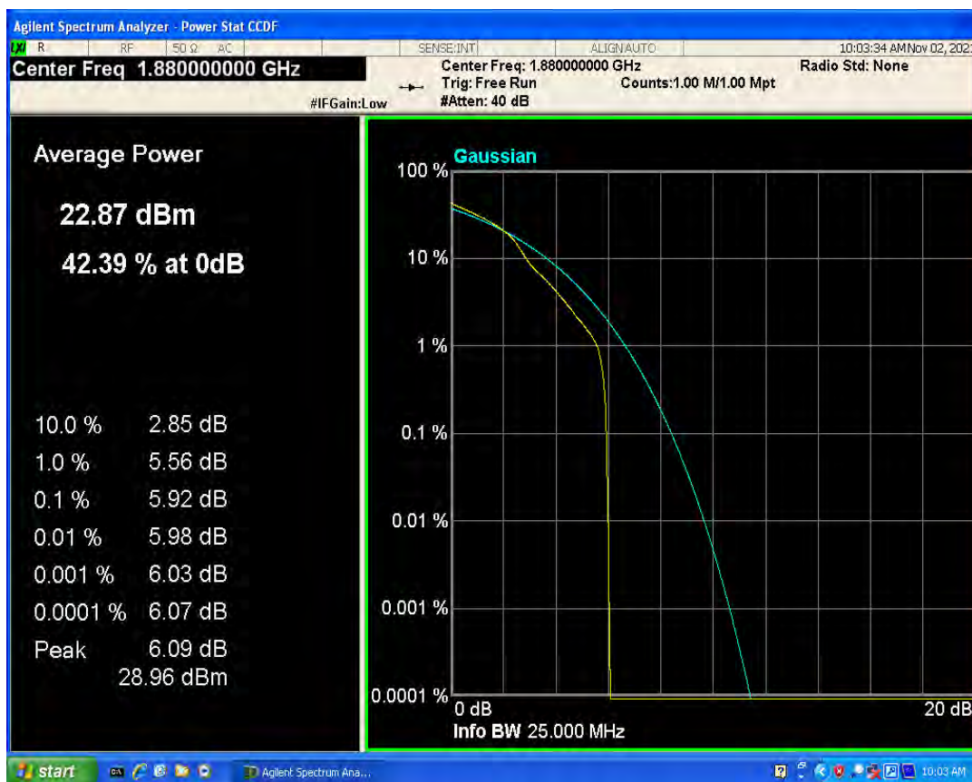
Band25 QPSK BW=1.4MHz Channel=26365 RB Size=1 Position=#0
