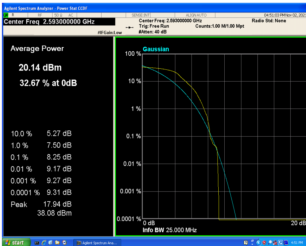
Band41 QAM16 BW=10MHz Channel=40620 RB Size=1 Position=#0
