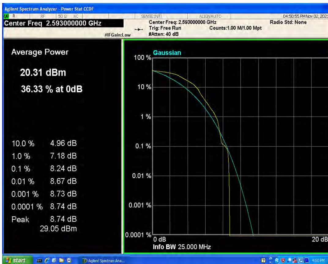
Band41 QPSK BW=10MHz Channel=40620 RB Size=1 Position=#0
