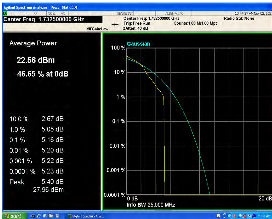
Band4 QPSK BW=20MHz Channel=20175 RB Size=1 Position=#0
