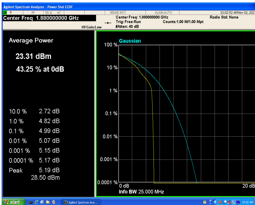
Band2 QAM16 BW=5MHz Channel=18900 RB Size=1 Position=#0
