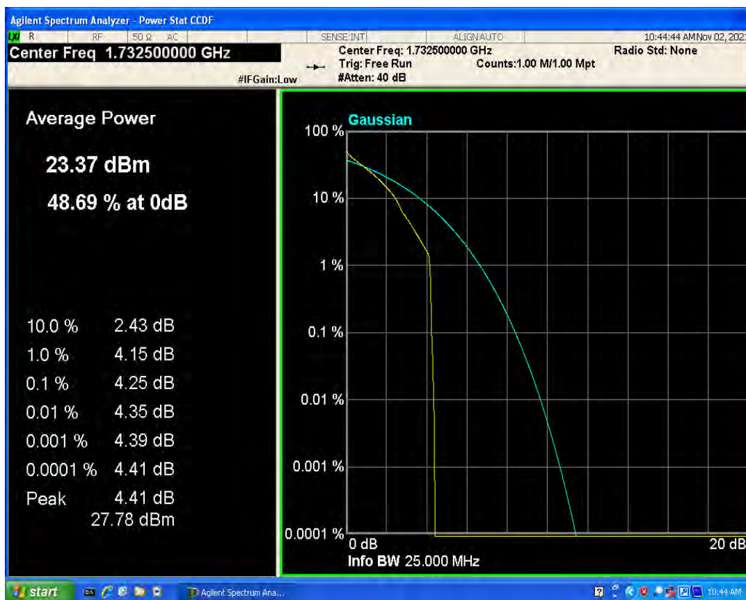
Band4 QAM16 BW=20MHz Channel=20175 RB Size=1 Position=#0
