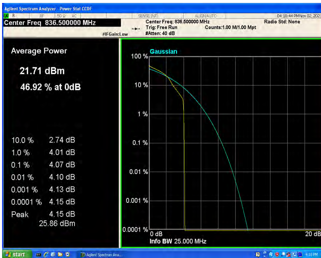
Band4 QPSK BW=1.4MHz Channel=20175 RB Size=1 Position=#0
