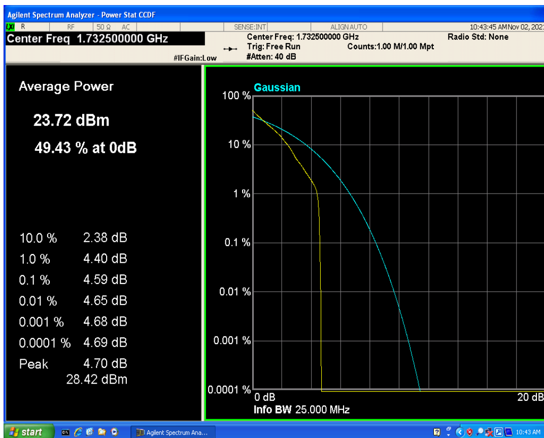
Band4 QAM16 BW=1.4MHz Channel=20175 RB Size=1 Position=#0
