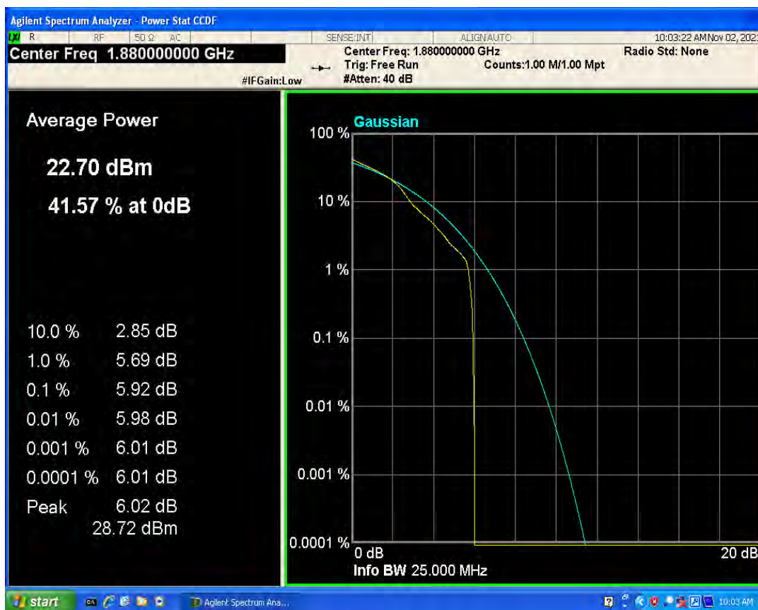
Band2 QPSK BW=20MHz Channel=18900 RB Size=1 Position=#0
