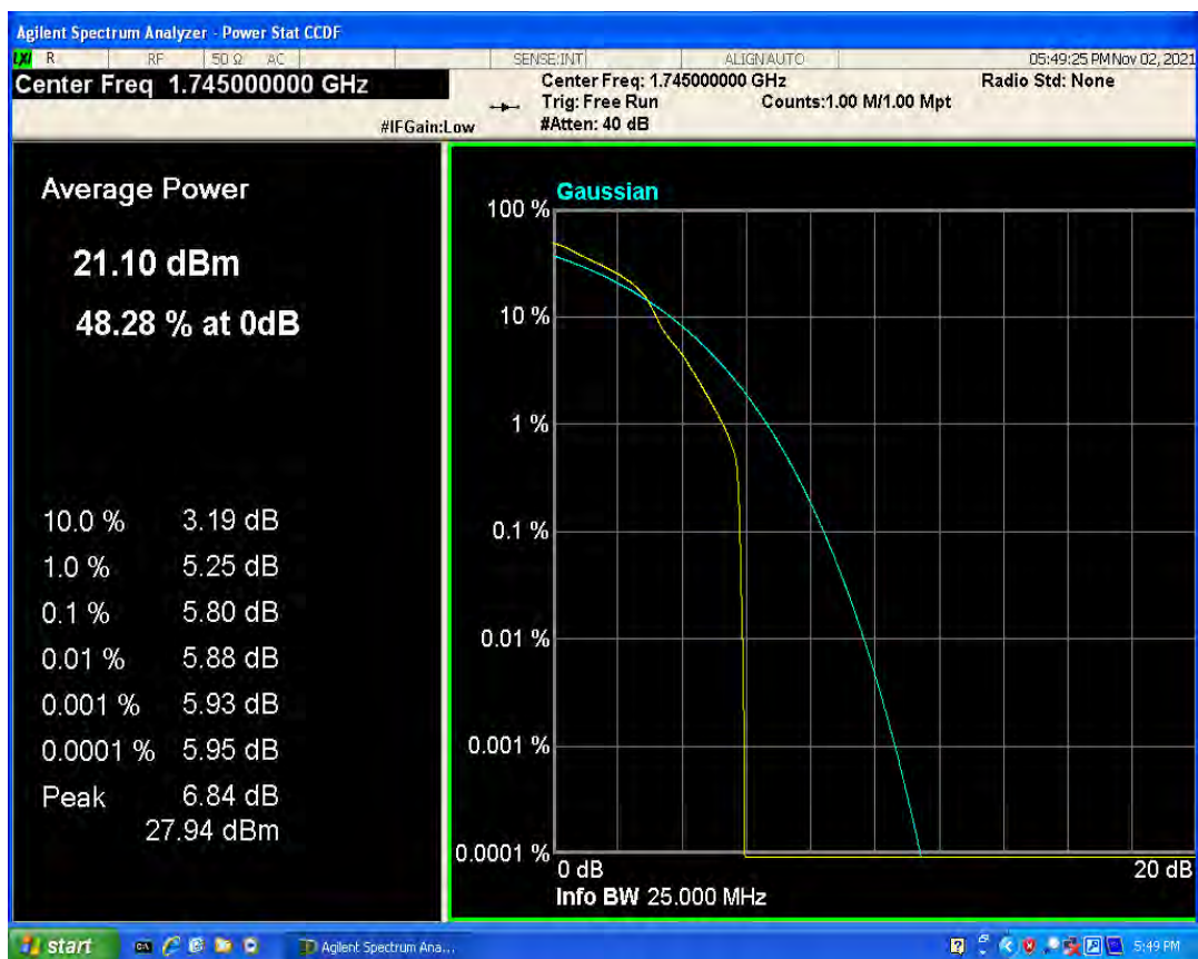
Band66 QPSK BW=20MHz Channel=132322 RB Size=1 Position=#0
