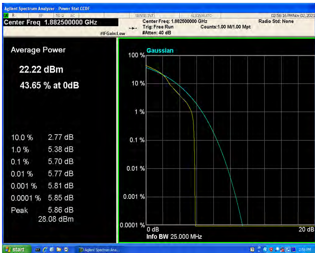
Band25 QPSK BW=10MHz Channel=26365 RB Size=1 Position=#0
