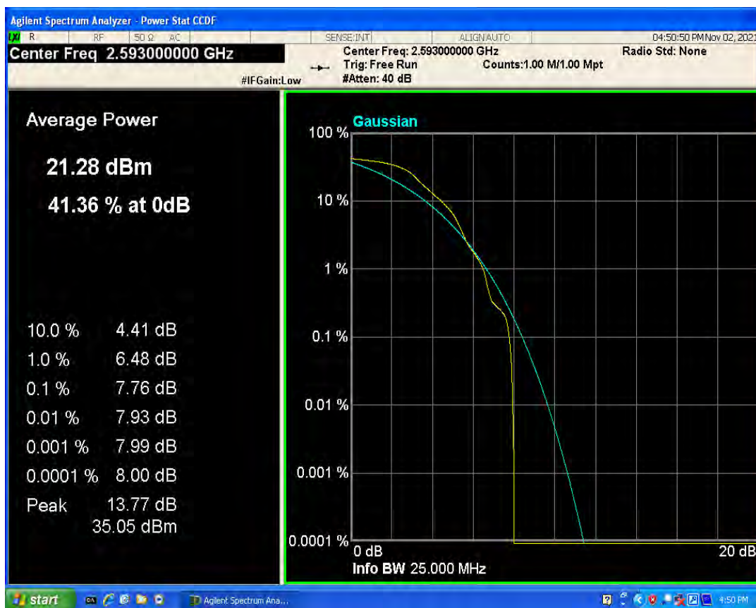
Band41 QAM16 BW=5MHz Channel=40620 RB Size=1 Position=#0
