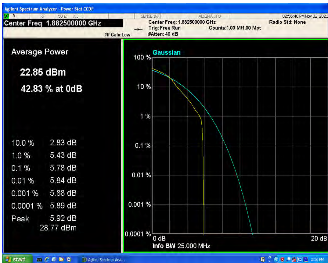
Band25 QPSK BW=20MHz Channel=26365 RB Size=1 Position=#0
