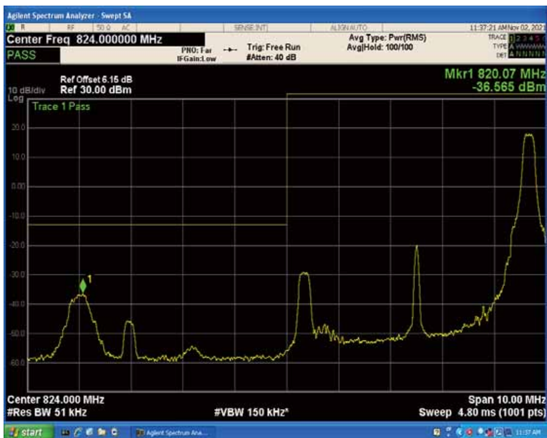
Band5 QAM16 BW=5MHz Channel=20425 RB Size=1 Position=#0
