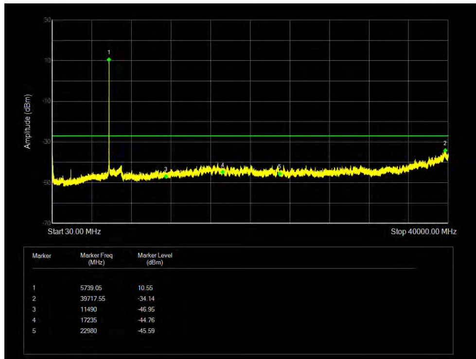
Tx. Spurious NVNT 802.11ac20 5745MHz Sum Emission
