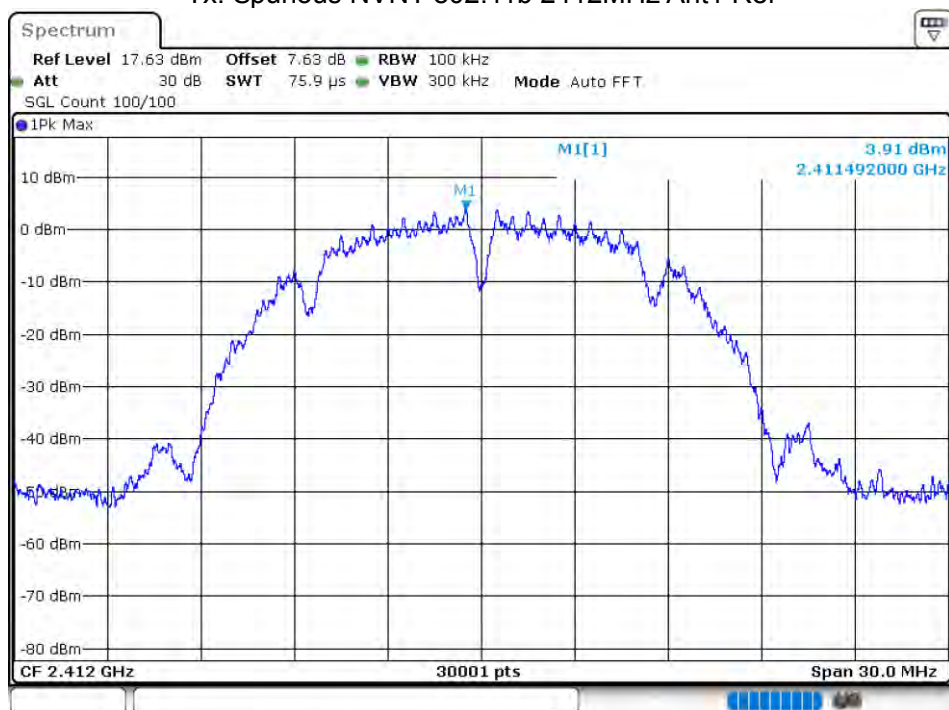
Tx. Spurious NVNT 802.11b 2412MHz Ant1 Ref
