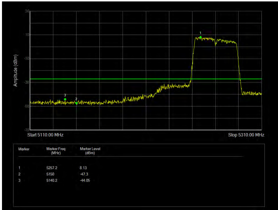
Band Edge NVNT 802.11n(HT40) 5310MHz High Ant 1
