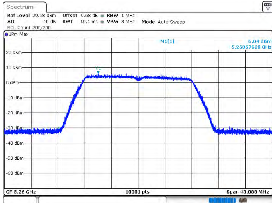
PSD NVNT 802.11n(HT20) 5260MHz Ant 2
