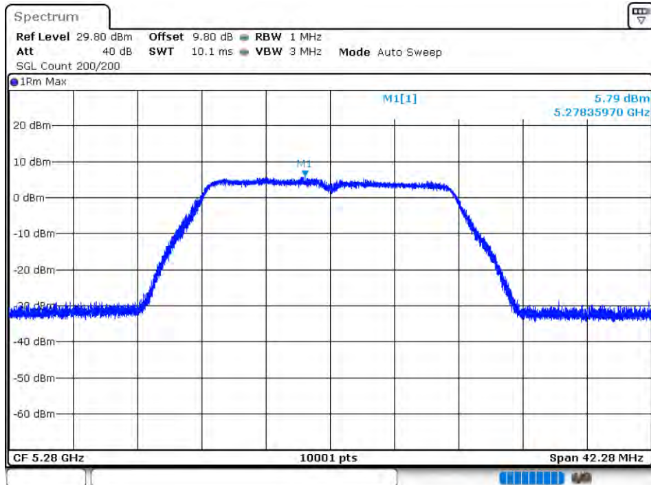
PSD NVNT 802.11a 5280MHz Ant 2
