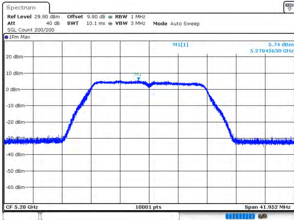
PSD NVNT 802.11a 5280MHz Ant 1
