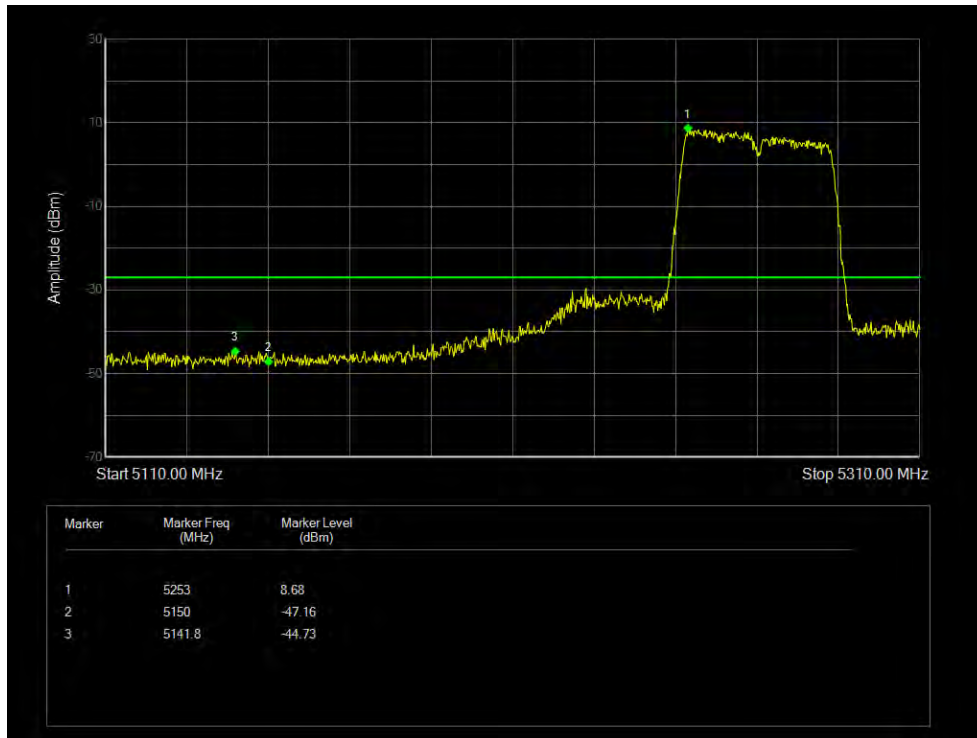
Band Edge NVNT 802.11n(HT40) 5310MHz High Ant 2
