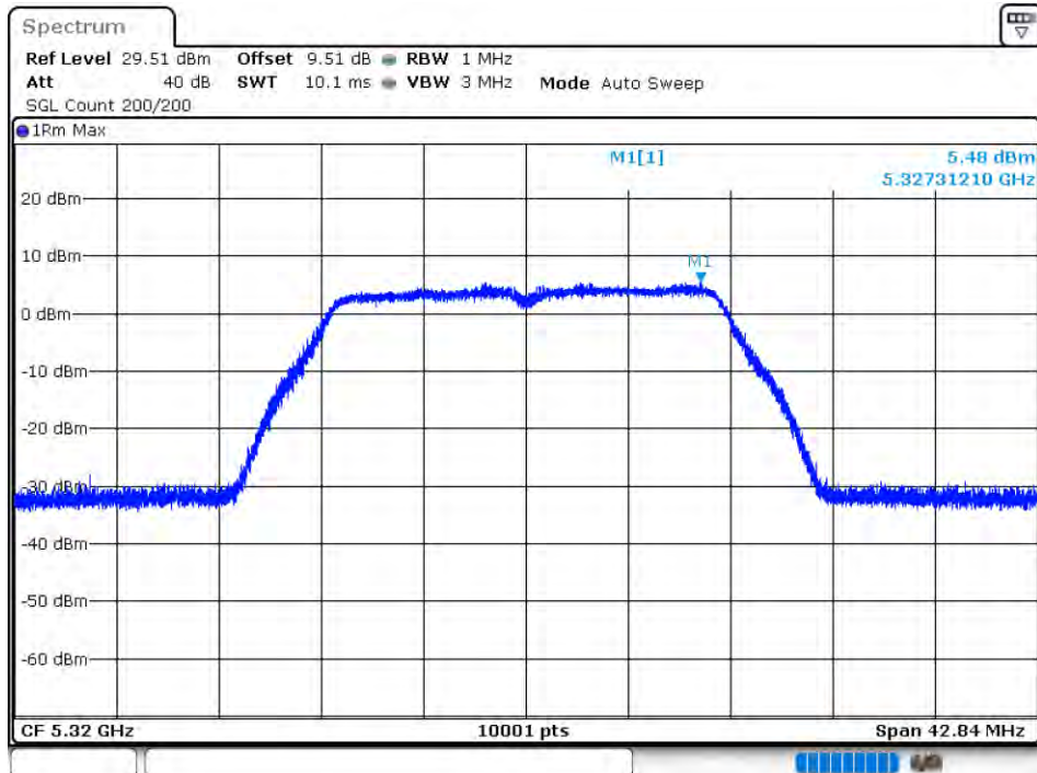
PSD NVNT 802.11a 5320MHz Ant 2
