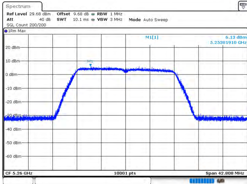
PSD NVNT 802.11n(HT20) 5260MHz Ant 1
