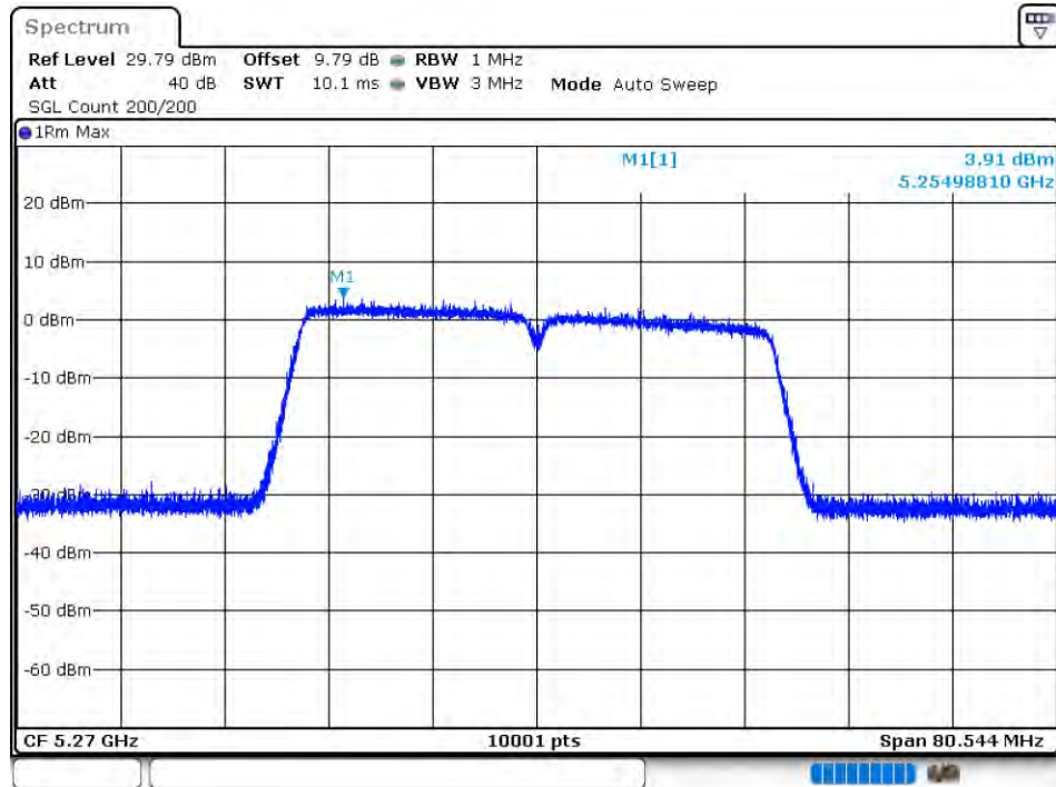
PSD NVNT 802.11n(HT40) 5270MHz Ant 1
