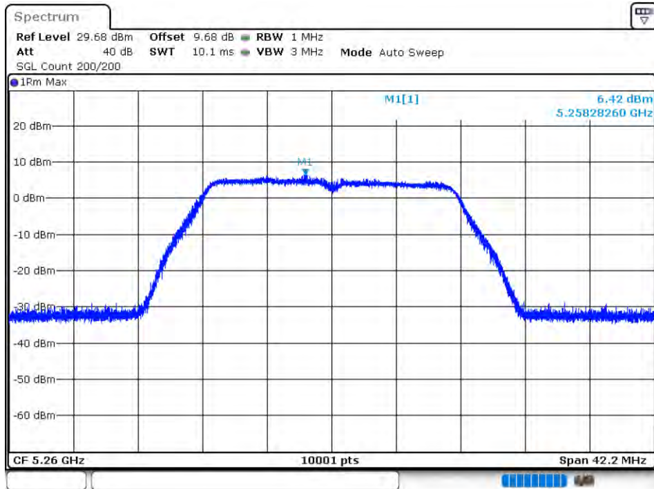
PSD NVNT 802.11a 5260MHz Ant 1
