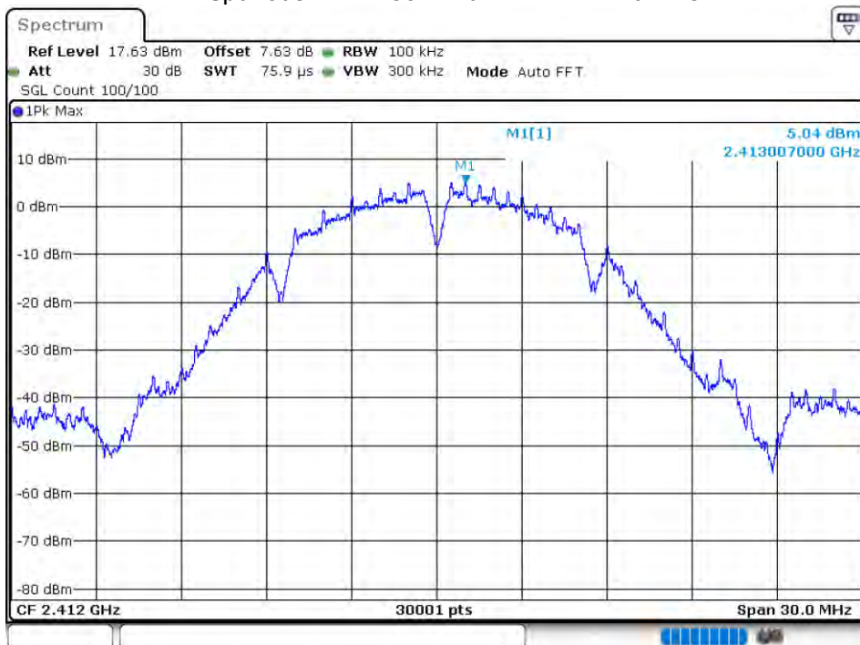
Tx. Spurious NVNT 802.11b 2412MHz Ant 1 Ref
