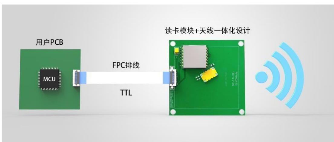
Figure 1-4 Three-wire connection, all tag information can be obtained by only one instruction.
