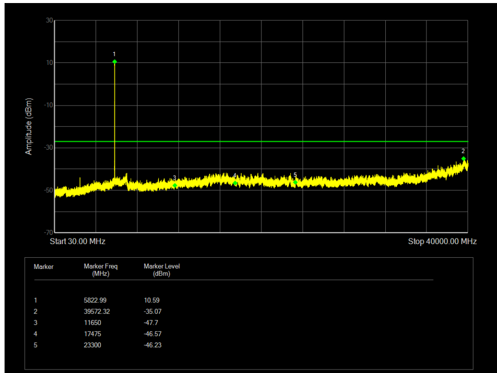
Tx. Spurious NVNT 802.11a 5825MHz Ant 2 Emission
