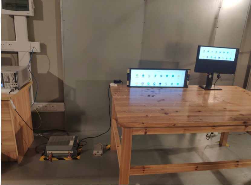
Photograph of test setup for Conducted Emission
