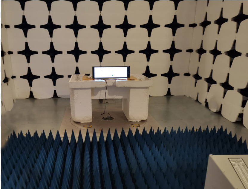
Photograph of test setup for Radiated Emission above 1 G
