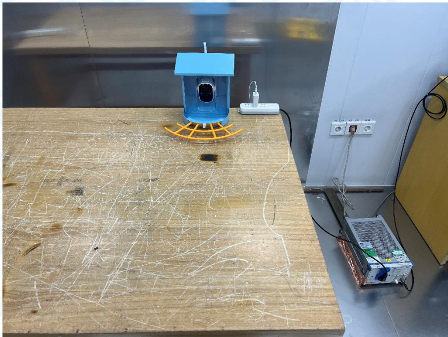
Photo of Setup for Conducted Emission
