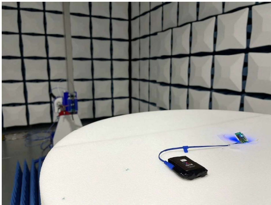
Set-up for Radiated Emission (1GHz above)
