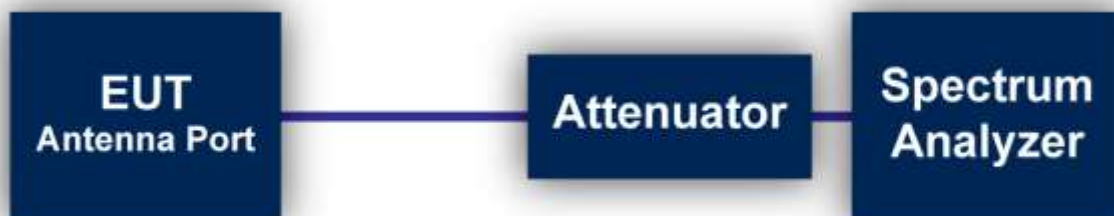
Figure 2: Direct Connection at the Antenna Port Test
