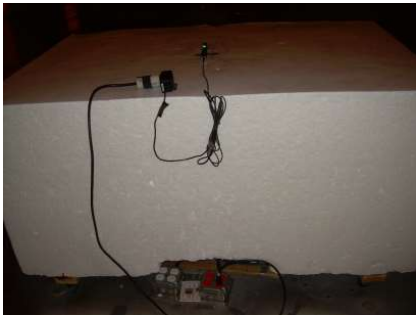
Photograph 2: Back View Radiated Emissions AC Mains Powered Flat Configuration – Below 1000 MHz
