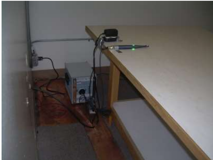
Photograph 8: Back View Conducted Emissions Worst-Case Configuration
