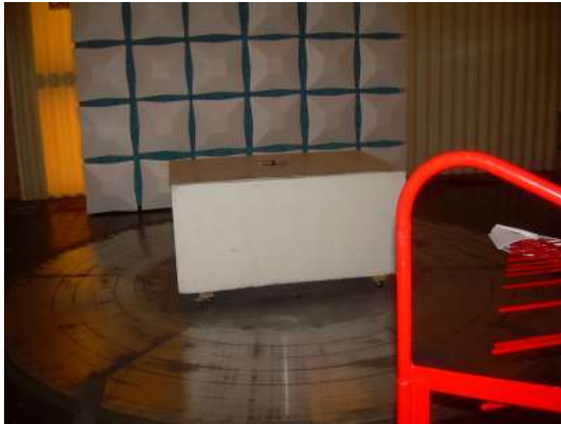
Photograph 1: Front View Radiated Emissions Battery Powered Flat Configuration – 30 – 1000 MHz
