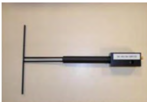
Figure 1 – Satimo COMOSAR Validation Dipole
