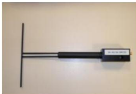
Figure 1 – Satimo COMOSAR Validation Dipole
