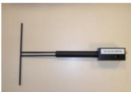
Figure 1 – Satimo COMOSAR Validation Dipole
