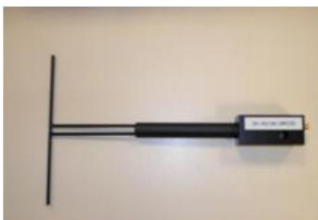
Figure 1 – Satimo COMOSAR Validation Dipole
