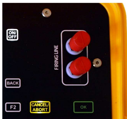
Figure 46. Firing line terminals
