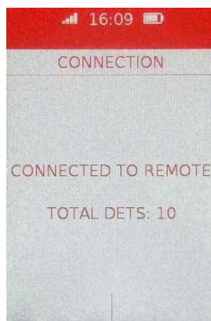
Figure 59. Blaster connected to Remote control device
