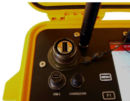
Figure 45. USB and charge sockets
