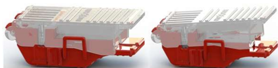
Figure 6. Completely Closed and half-closed connectors
