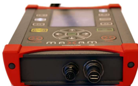
Figure 80. USB and charge sockets
