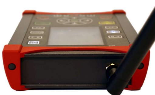
Figure 81. Communication antenna socket
