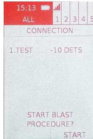
Figure 85. Remote is ready to start blast procedure
