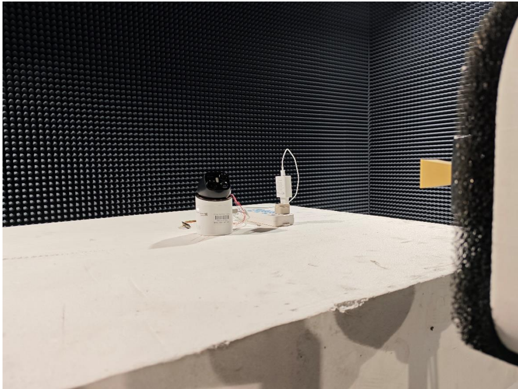
Photograph 3: Set-up for Conducted Emission on AC Mains
