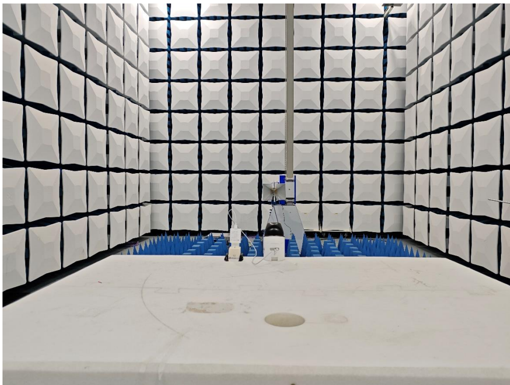
Photograph 2: Set-up for Radiated Spurious Emission, Above 1GHz
