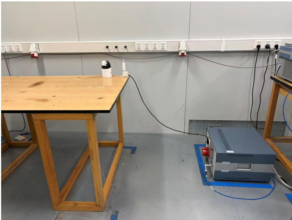
Photograph 3: Set-up for Conducted Emission on AC Mains
