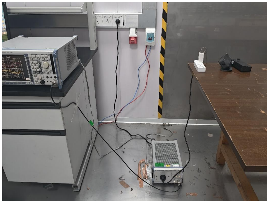
Conducted Emission Test Setup
