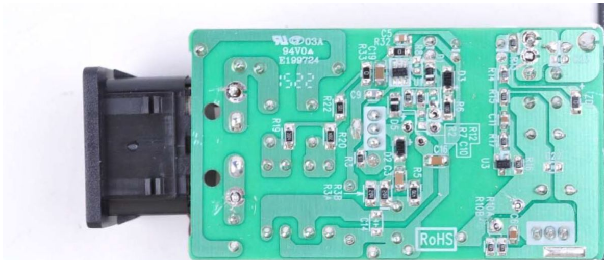
PCB inside the AC adaptor (Bottom)
