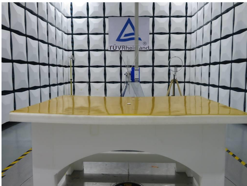
Photograph 1: Set-up photo for Radiated Spurious Emission, Below 1GHz
