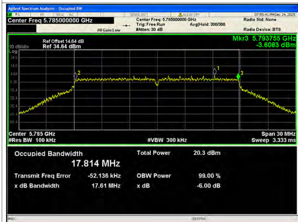
-6dB Bandwidth NVNT ac20 5785MHz Ant2 MIMO
