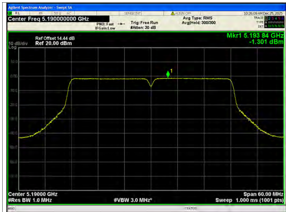
PSD NVNT ac40 5190MHz Ant1 MIMO
