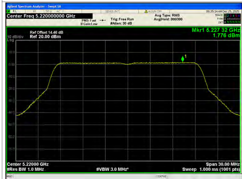
PSD NVNT be20 5220MHz Ant2 MIMO
