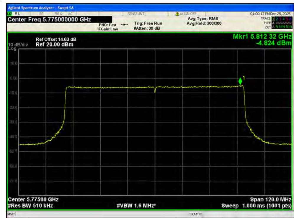
PSD NVNT be80 5775MHz Ant2 MIMO
