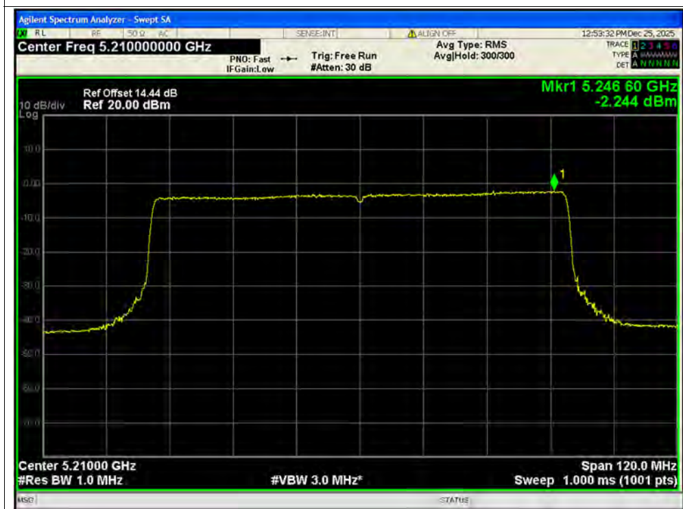
PSD NVNT ax80 5210MHz Ant2 MIMO
