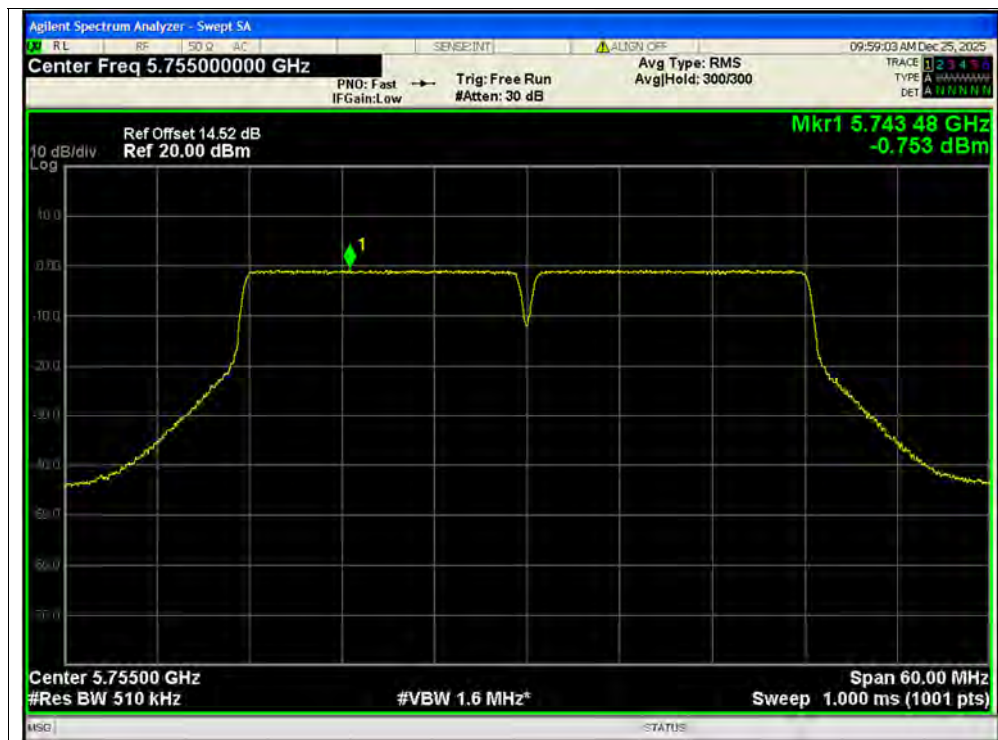
PSD NVNT ac40 5755MHz Ant2 SISO
