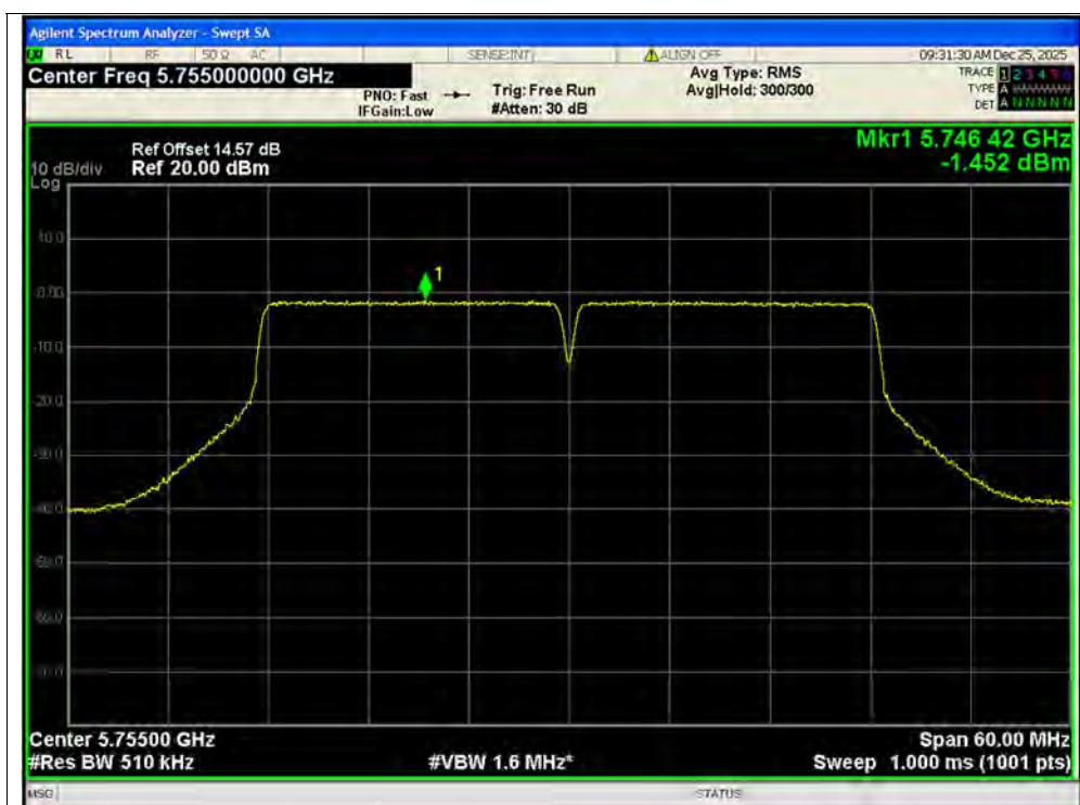
PSD NVNT ac40 5755MHz Ant1 SISO
