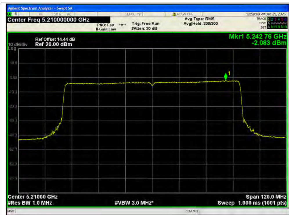
PSD NVNT be80 5210MHz Ant2 MIMO
