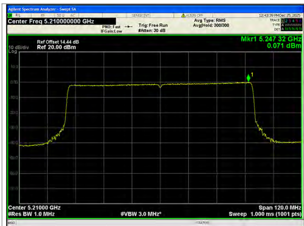
PSD NVNT be80 5210MHz Ant2 SISO
