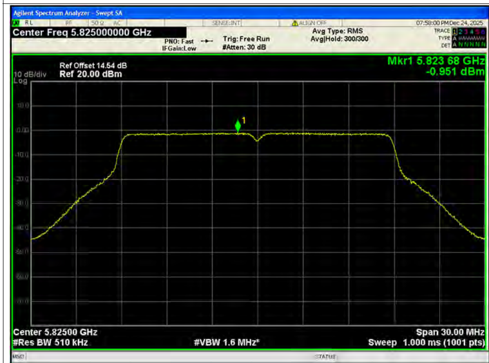
PSD NVNT ac20 5825MHz Ant2 MIMO
