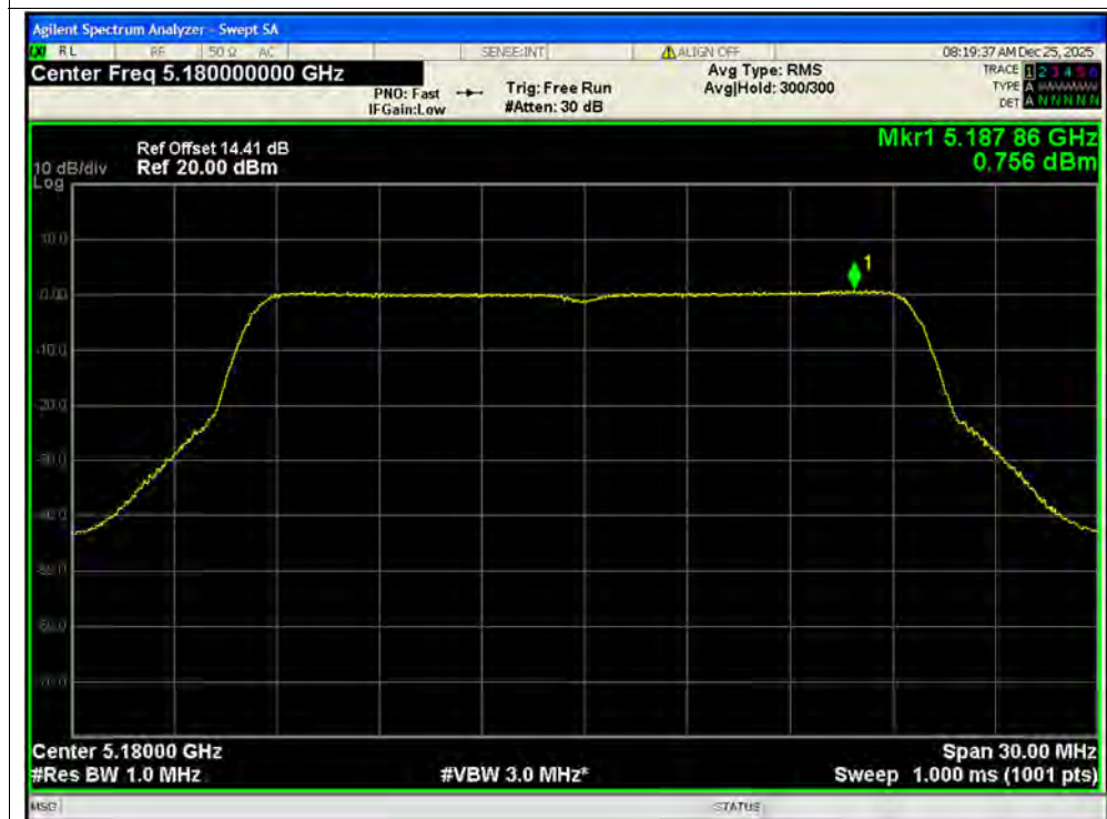
PSD NVNT ax20 5180MHz Ant2 MIMO
