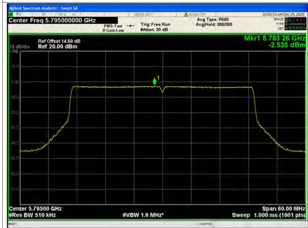
PSD NVNT be40 5795MHz Ant2 MIMO
