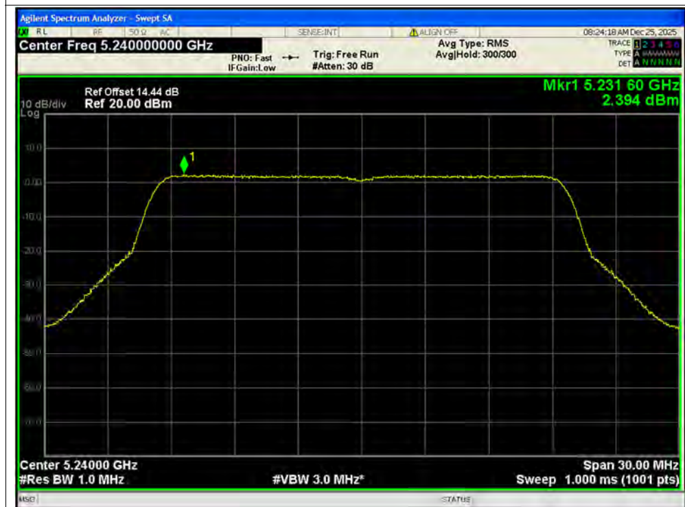
PSD NVNT ax20 5240MHz Ant2 MIMO
