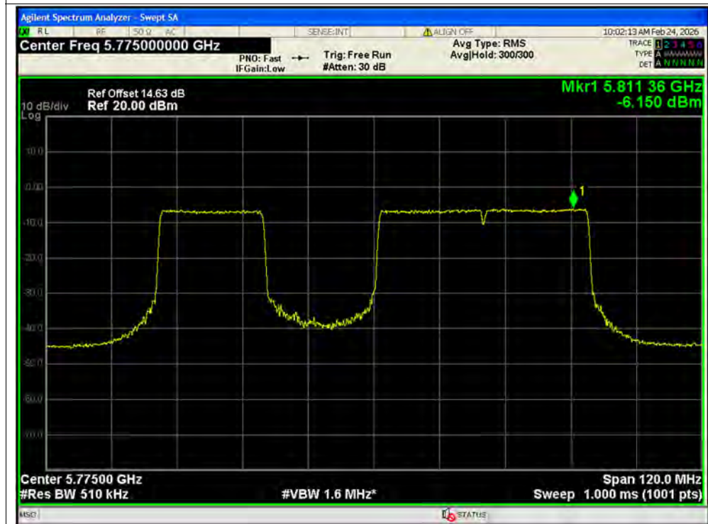
PSD NVNT be80 puncturing 20 MRU2 5775MHz Ant2 MIMO
