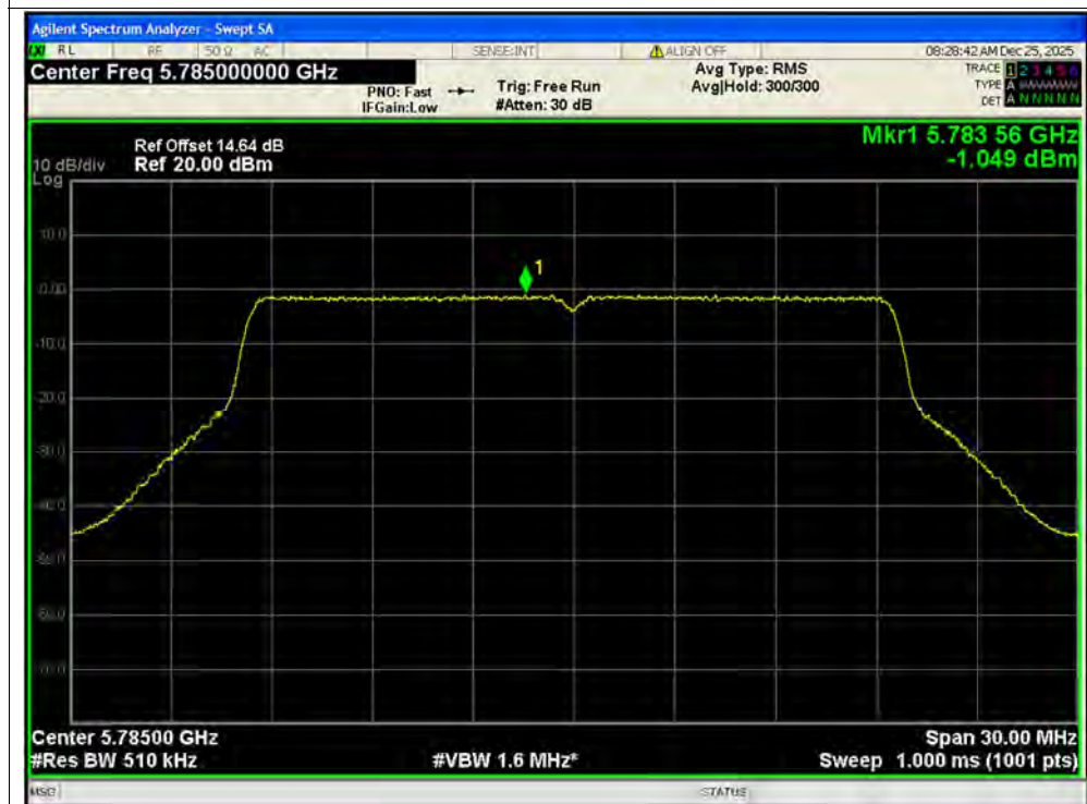
PSD NVNT ax20 5785MHz Ant2 MIMO
