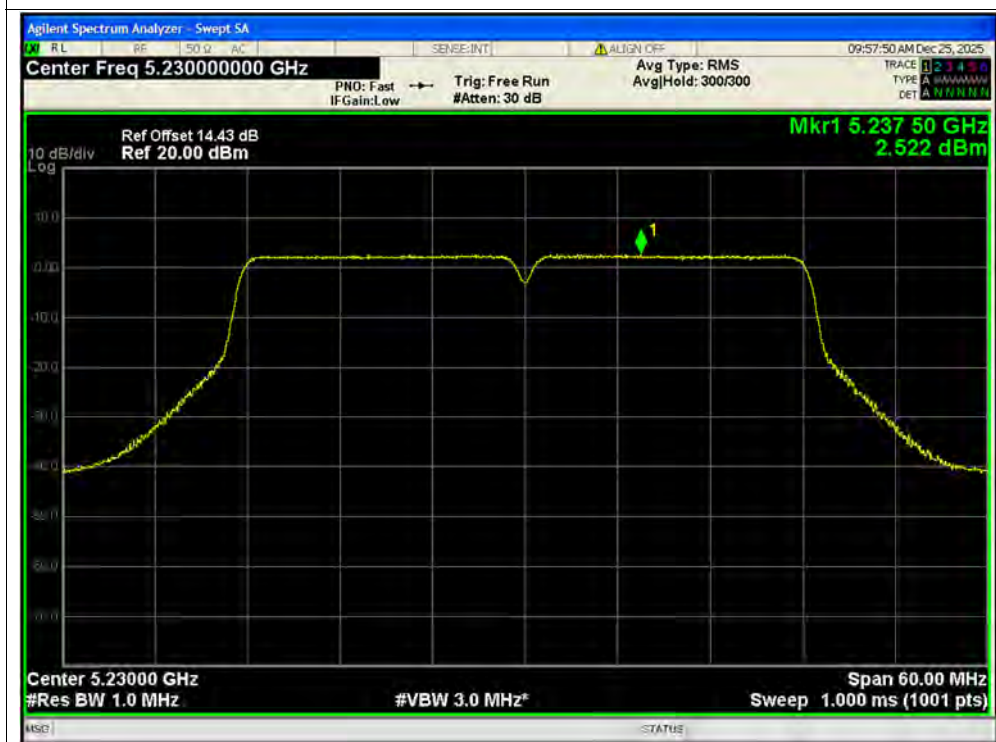
PSD NVNT ac40 5230MHz Ant2 SISO
