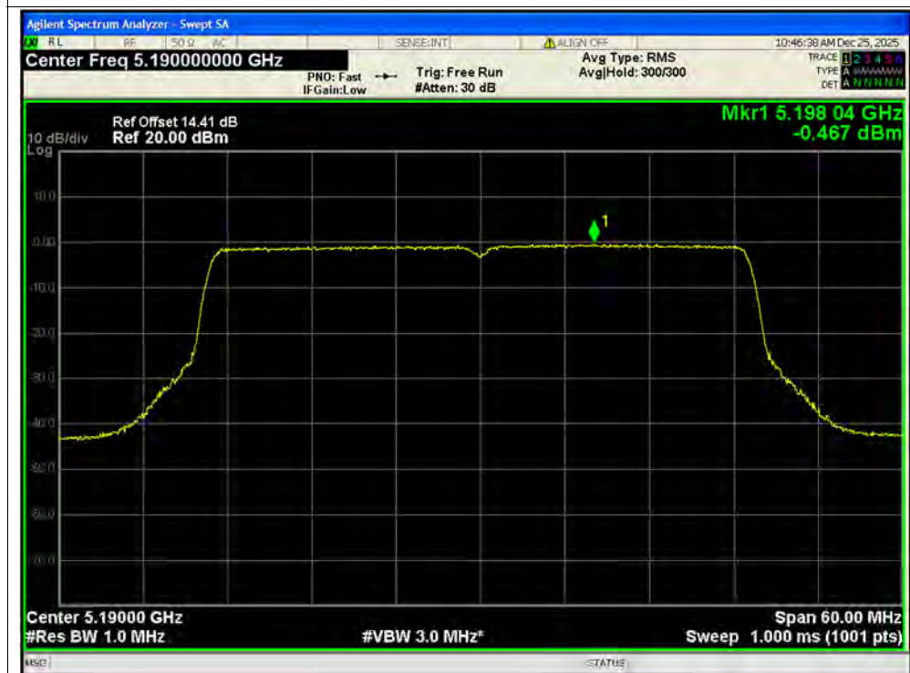
PSD NVNT be40 5190MHz Ant2 MIMO
