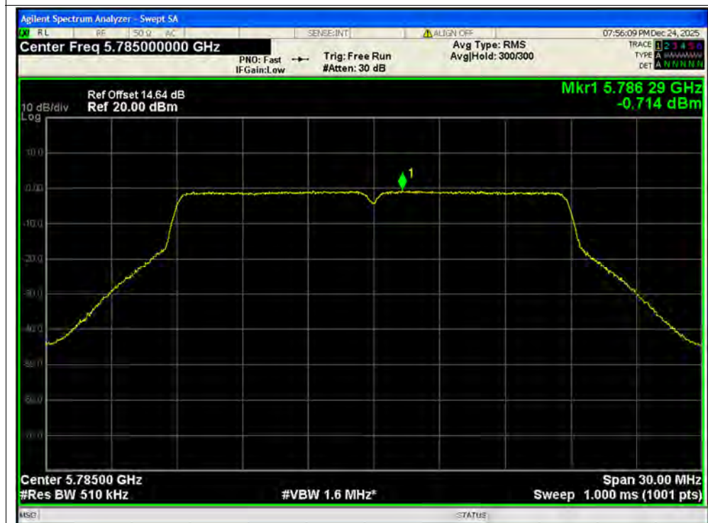
PSD NVNT ac20 5785MHz Ant2 MIMO
