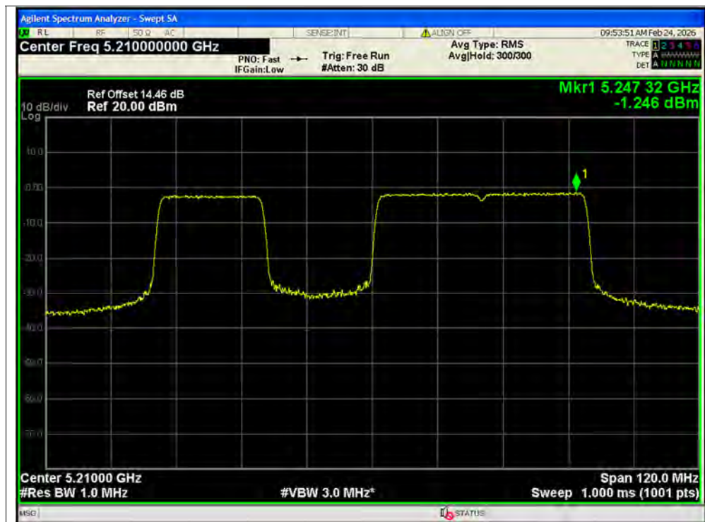
PSD NVNT be80 puncturing 20 MRU2 5210MHz Ant1 SISO
