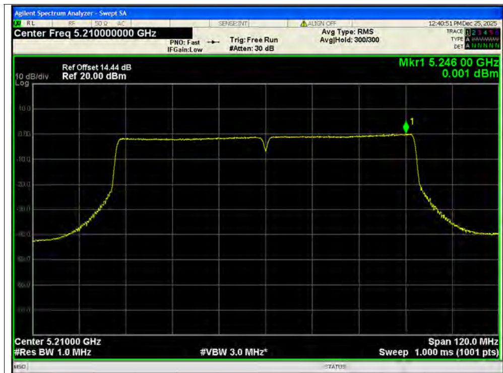
PSD NVNT ac80 5210MHz Ant2 SISO
