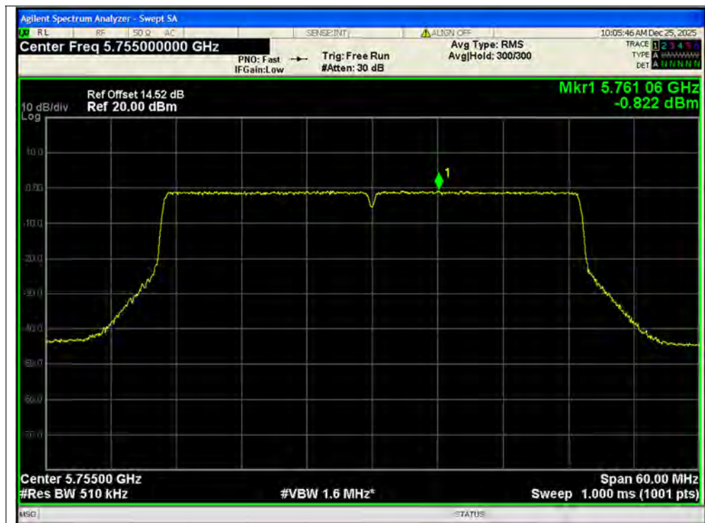
PSD NVNT ax40 5755MHz Ant2 SISO
