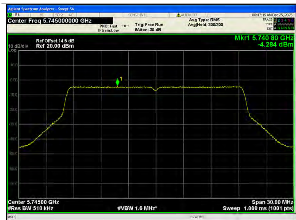
PSD NVNT be20 5745MHz Ant1 MIMO
