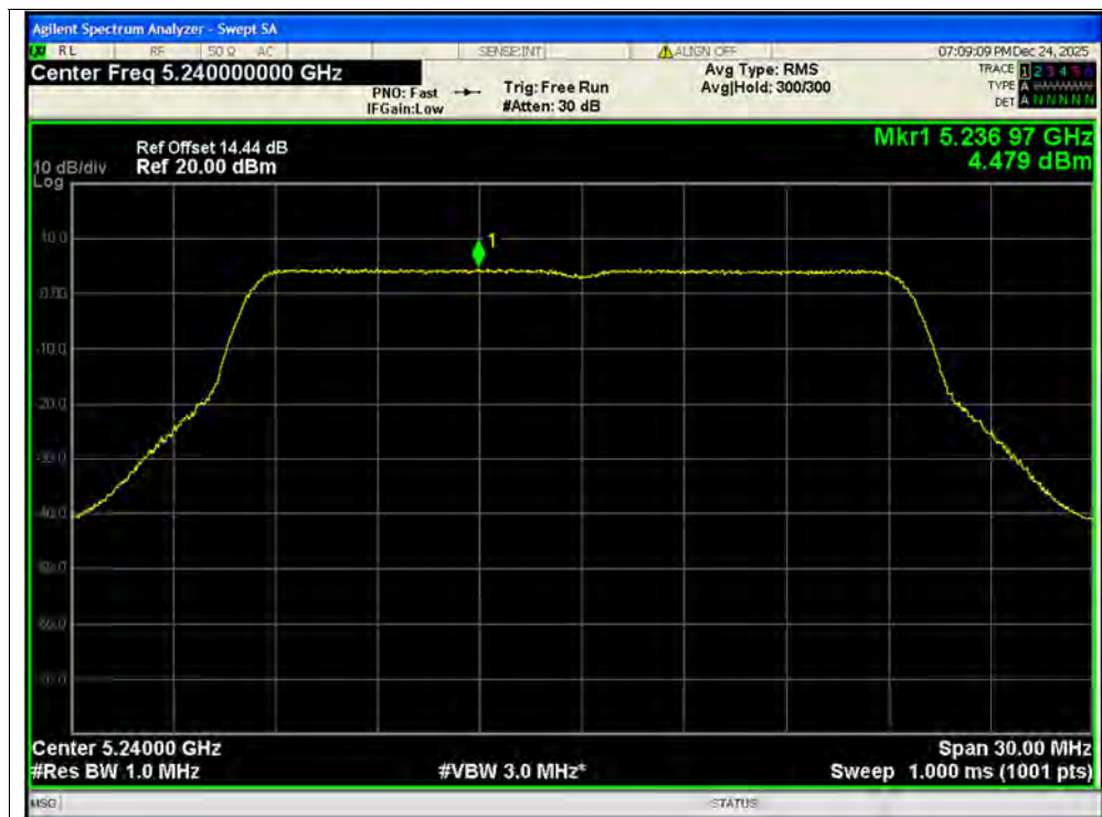
PSD NVNT ax20 5240MHz Ant2 SISO
