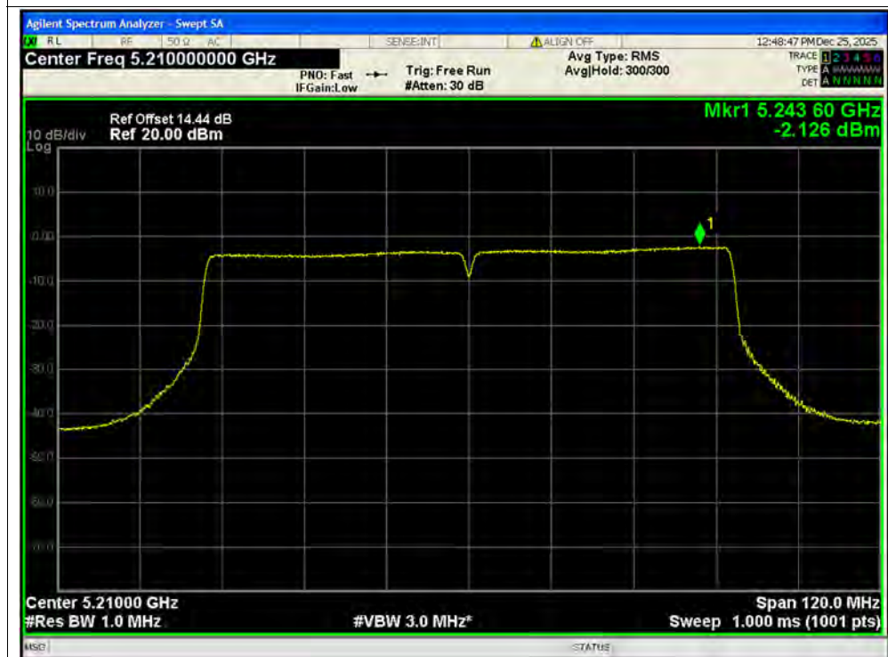
PSD NVNT ac80 5210MHz Ant2 MIMO
