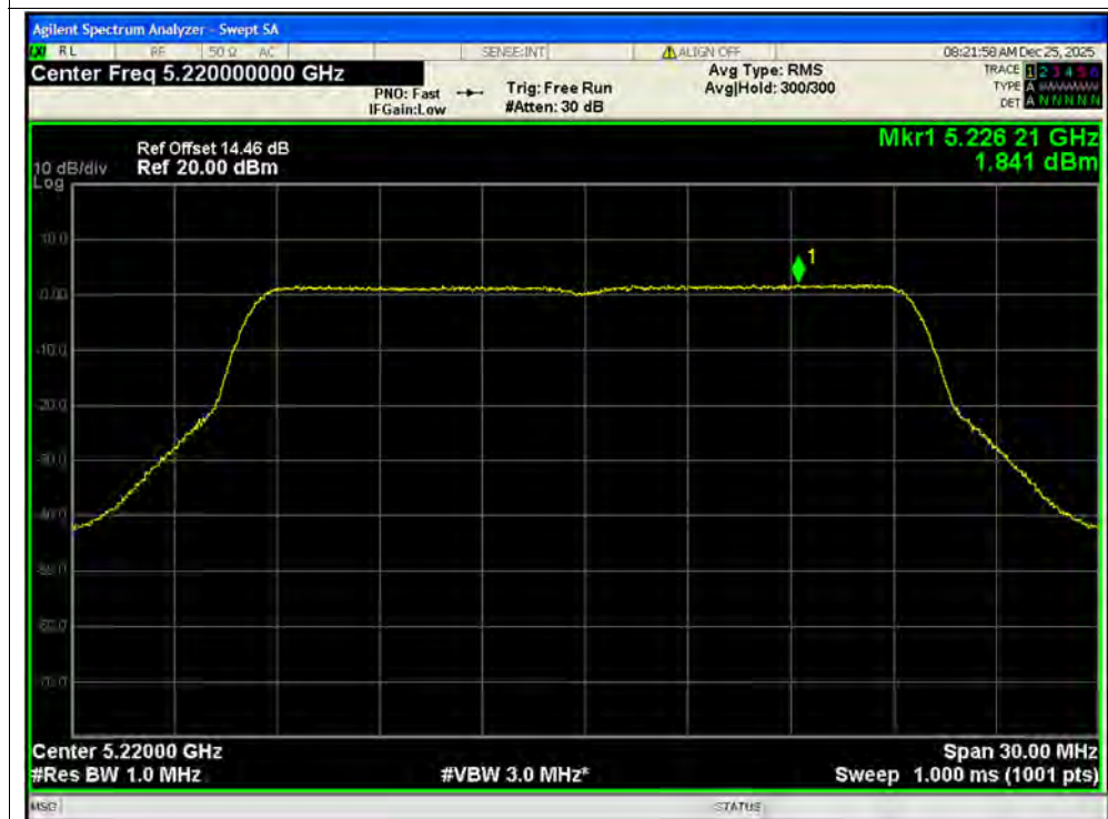
PSD NVNT ax20 5220MHz Ant2 MIMO
