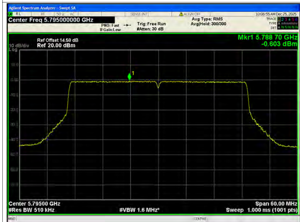
PSD NVNT ax40 5795MHz Ant2 SISO
