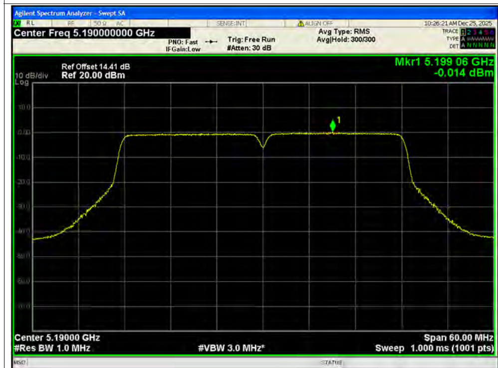
PSD NVNT ac40 5190MHz Ant2 MIMO
