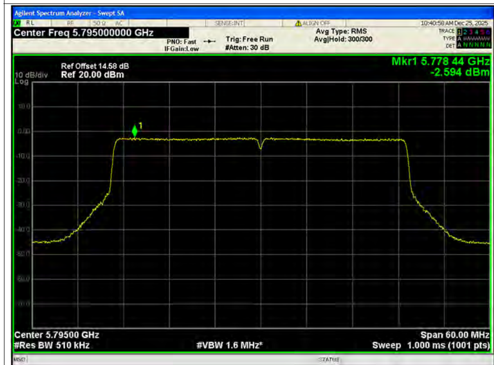
PSD NVNT ax40 5795MHz Ant2 MIMO
