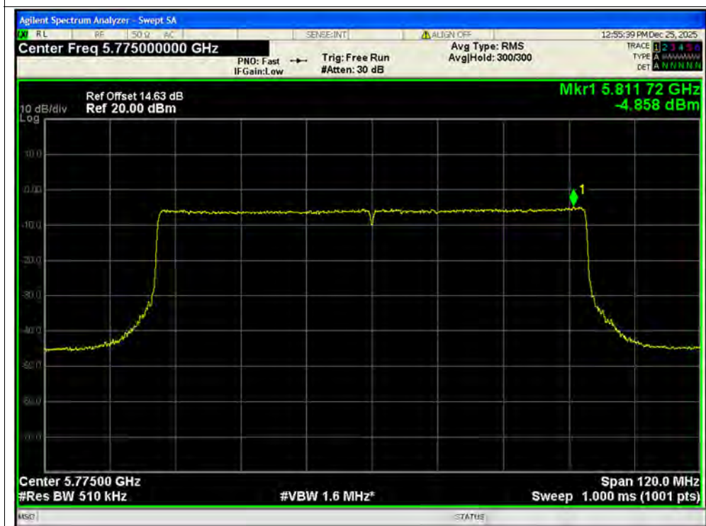
PSD NVNT ax80 5775MHz Ant2 MIMO
