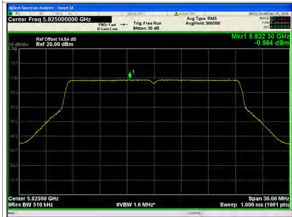
PSD NVNT be20 5825MHz Ant2 MIMO
