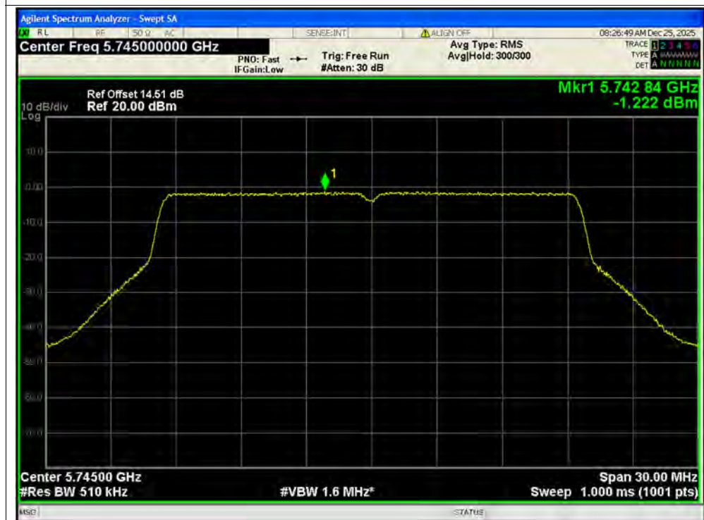
PSD NVNT ax20 5745MHz Ant2 MIMO
