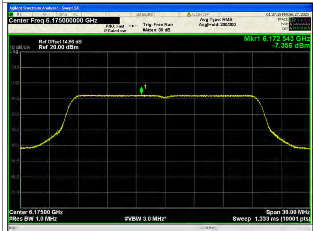
PSD NVNT ax20 6175MHz Ant2 SISO
