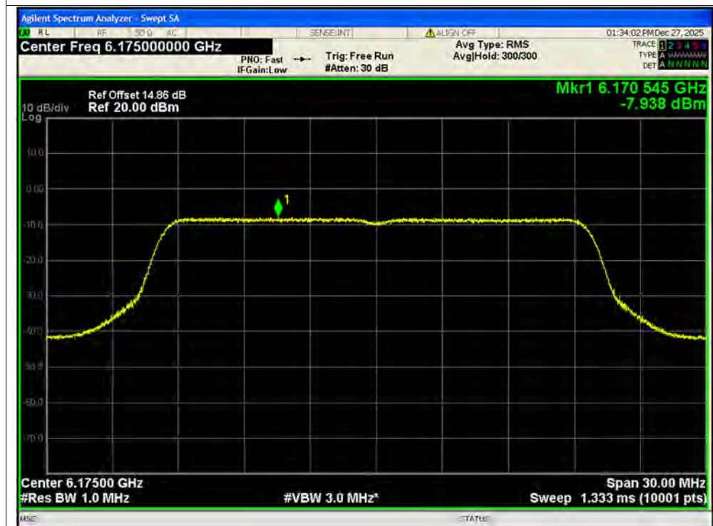
PSD NVNT ax20 6175MHz Ant2 MIMO
