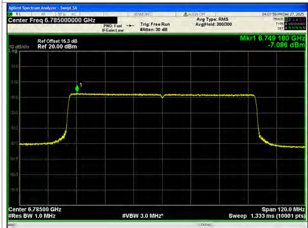
PSD NVNT ax80 6785MHz Ant2 SISO
