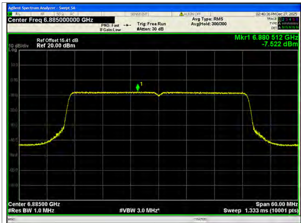
PSD NVNT ax40 6885MHz Ant1 SISO
