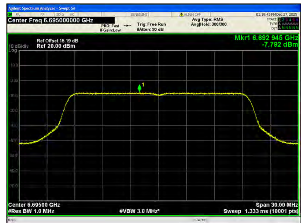
PSD NVNT ax20 6695MHz Ant2 SISO
