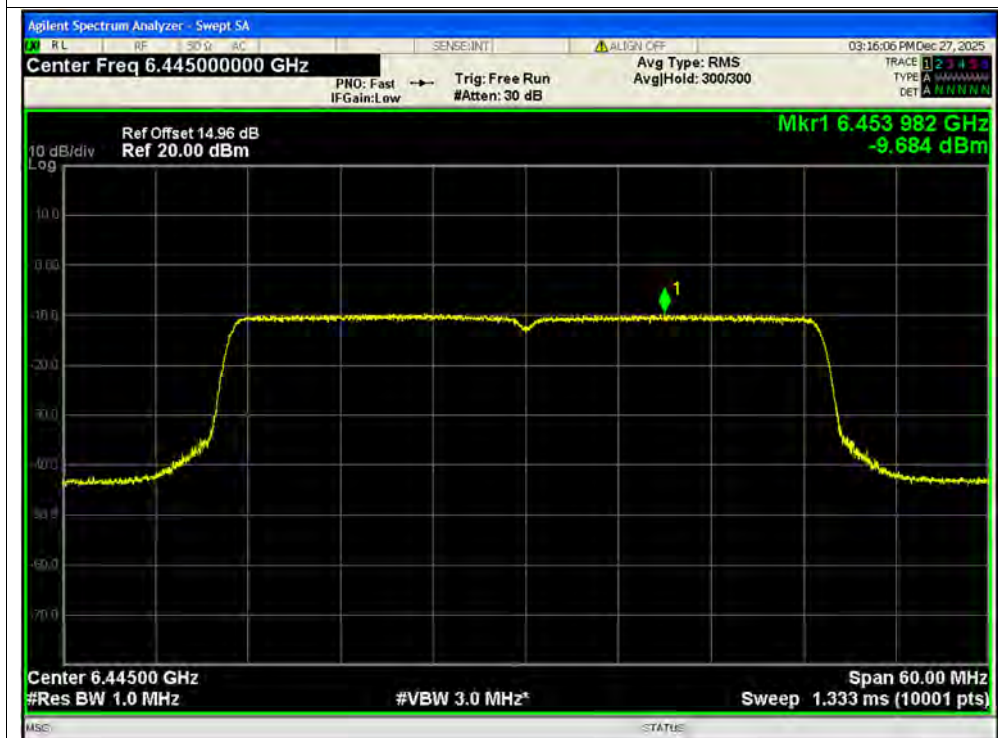
PSD NVNT ax40 6445MHz Ant2 MIMO
