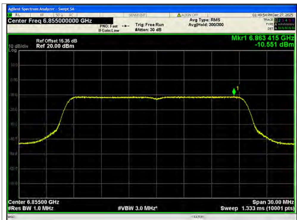
PSD NVNT ax20 6855MHz Ant1 MIMO
