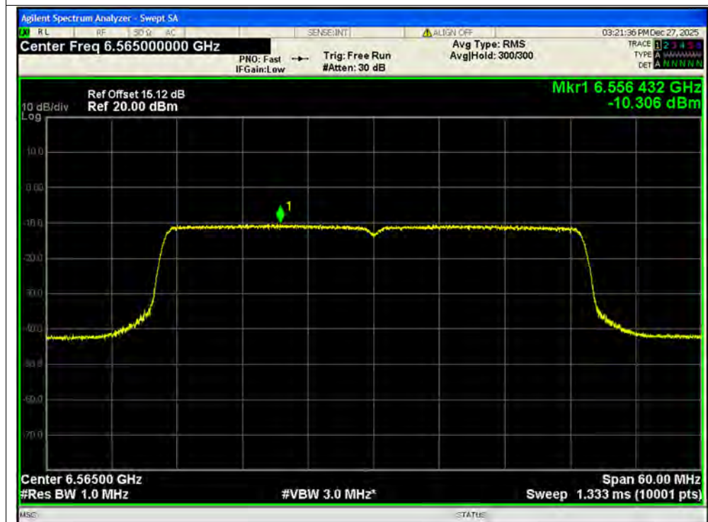
PSD NVNT ax40 6565MHz Ant2 MIMO
