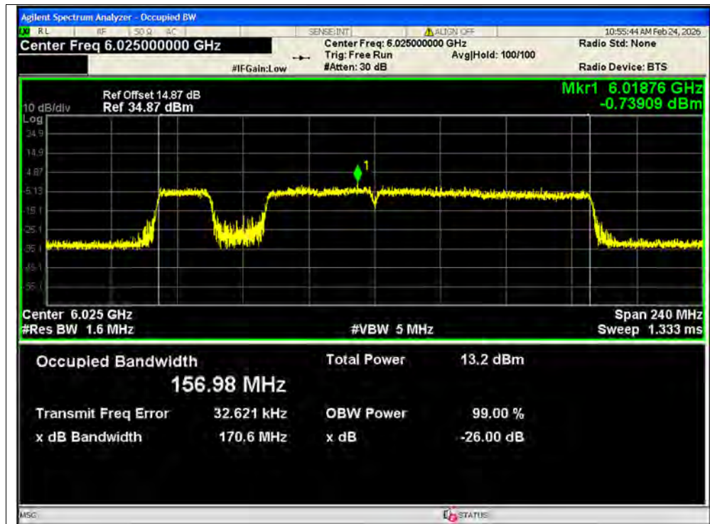
OBW NVNT be160 puncturing 20 MRU2 6025MHz Ant1 MIMO
