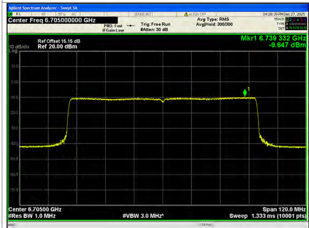
PSD NVNT ax80 6705MHz Ant2 MIMO
