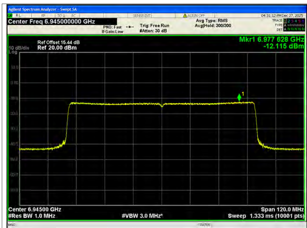
PSD NVNT ax80 6945MHz Ant1 MIMO
