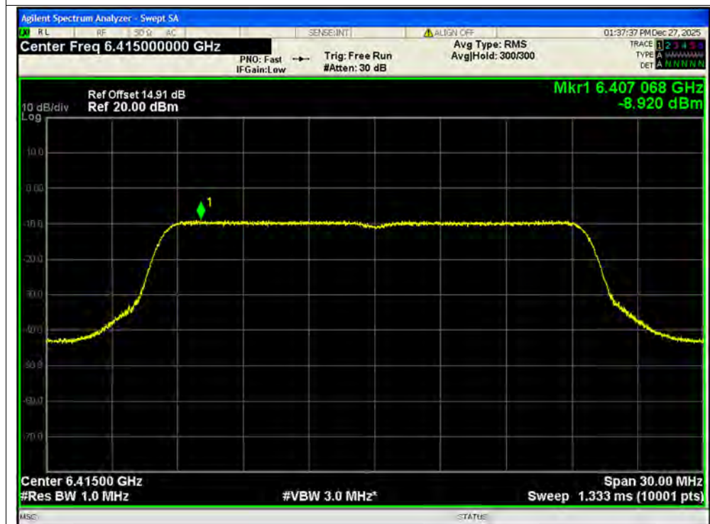
PSD NVNT ax20 6415MHz Ant2 MIMO
