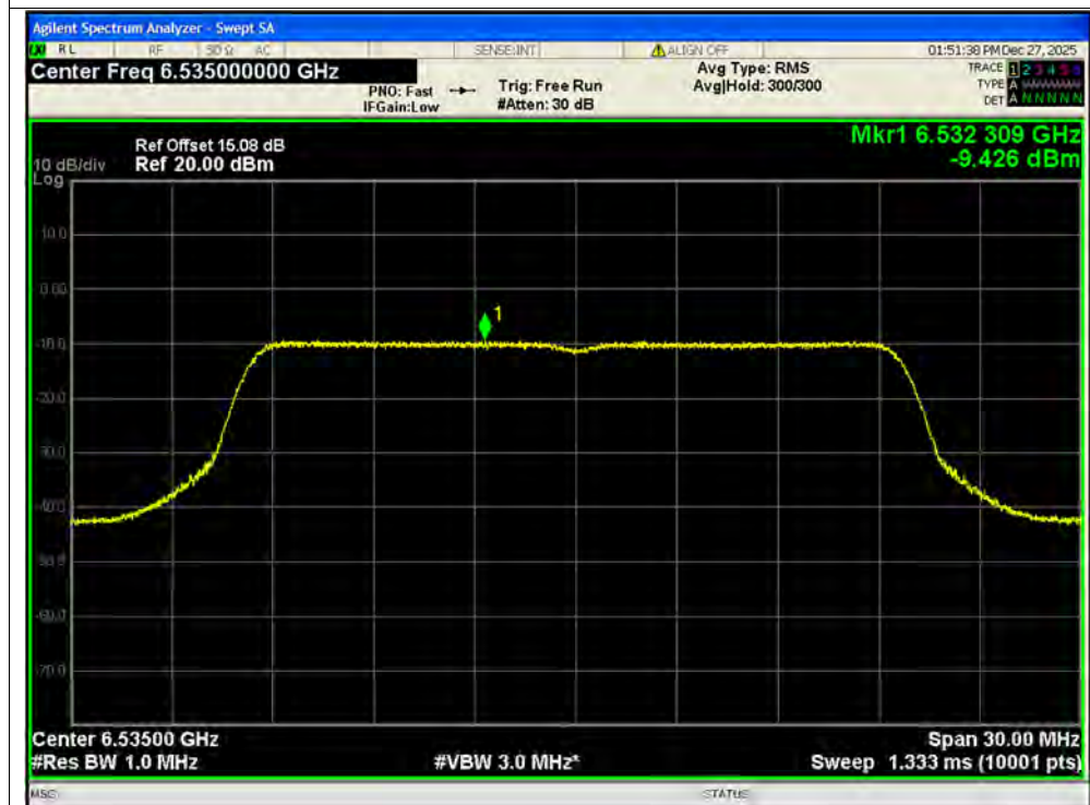
PSD NVNT ax20 6535MHz Ant2 MIMO
