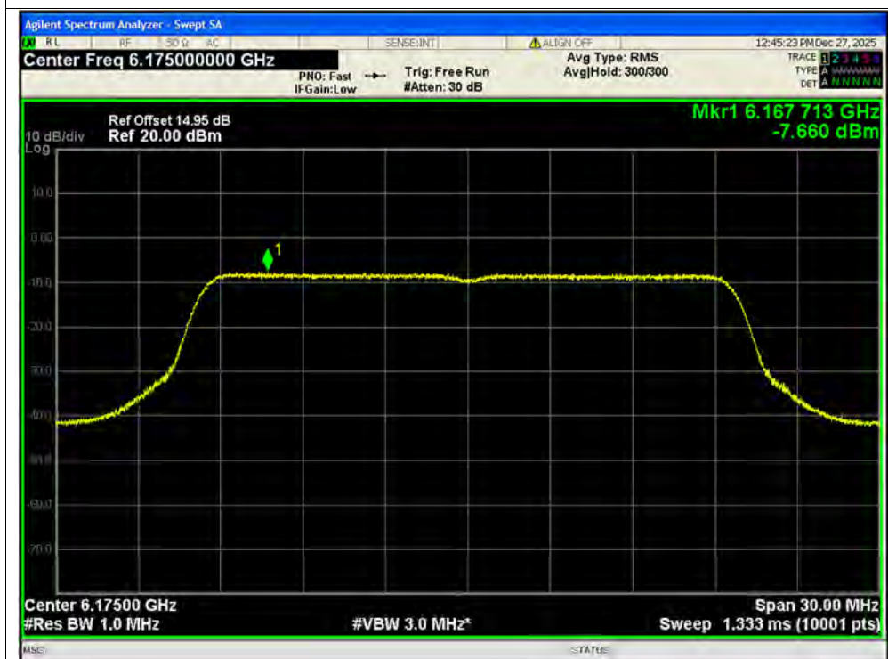
PSD NVNT be20 6175MHz Ant1 SISO
