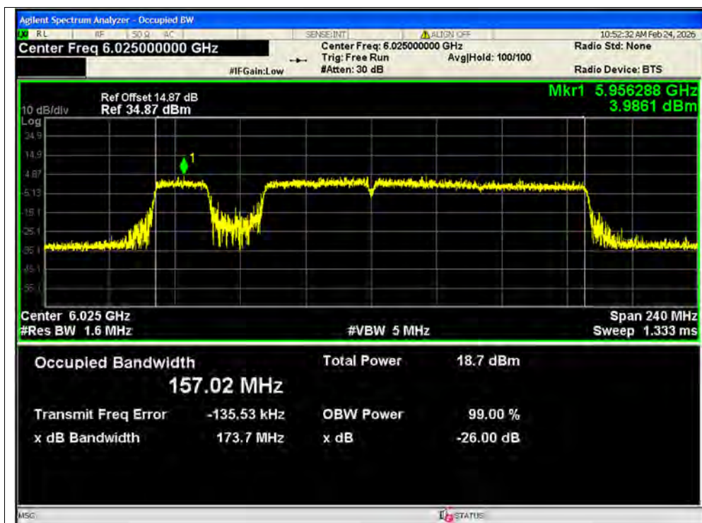
OBW NVNT be160 puncturing 20 MRU2 6025MHz Ant1 SISO
