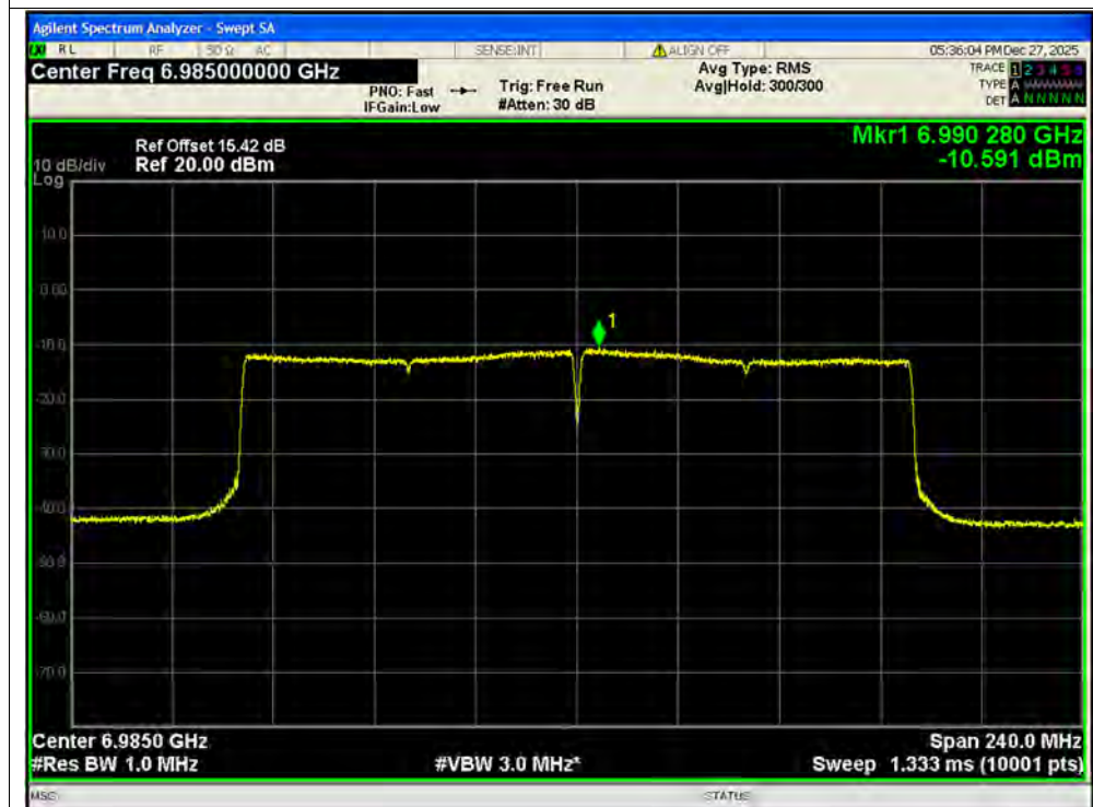
PSD NVNT ax160 6985MHz Ant2 MIMO
