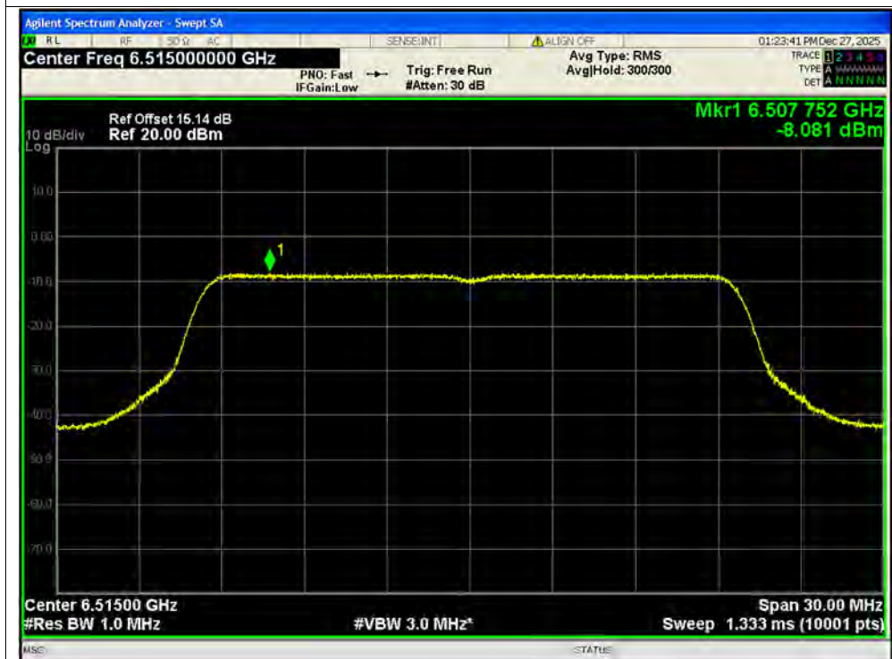
PSD NVNT be20 6515MHz Ant2 SISO
