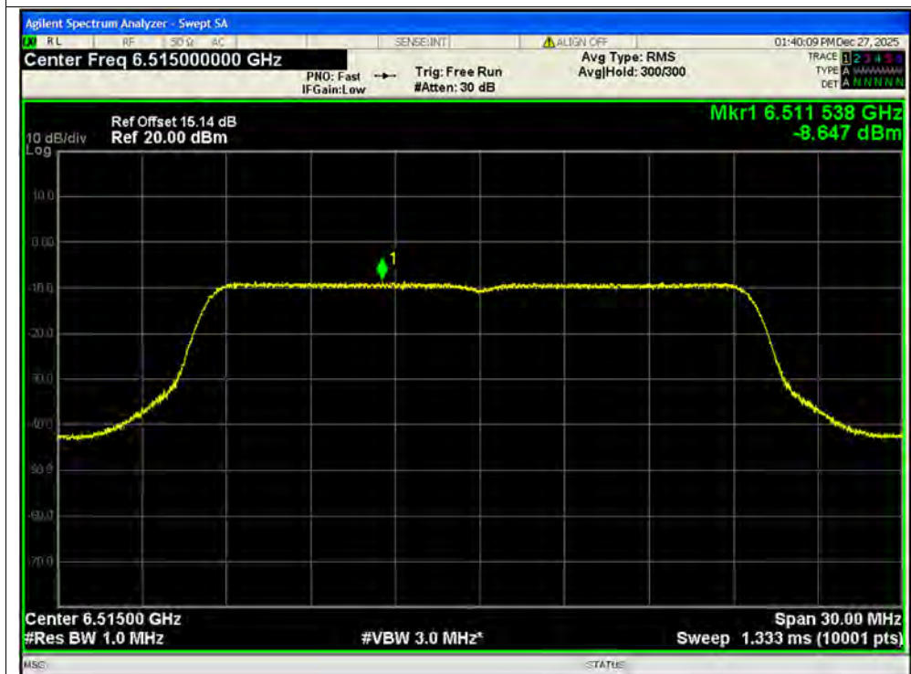
PSD NVNT ax20 6515MHz Ant2 MIMO
