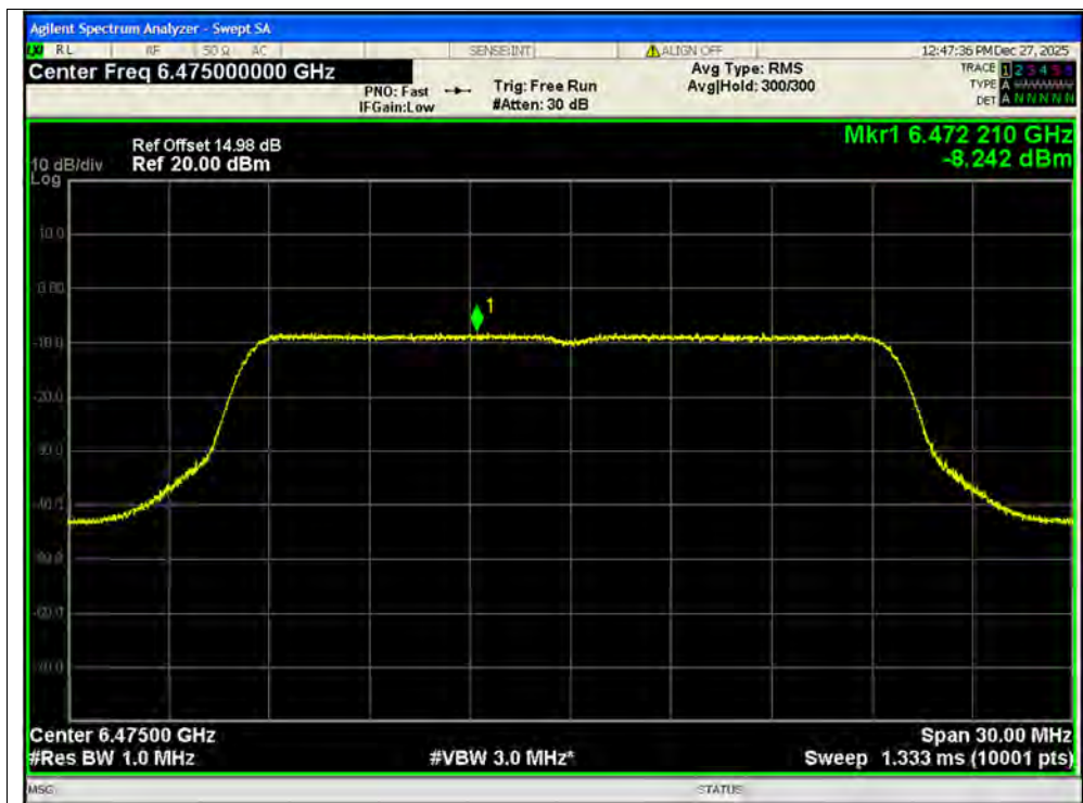
PSD NVNT be20 6475MHz Ant1 SISO
