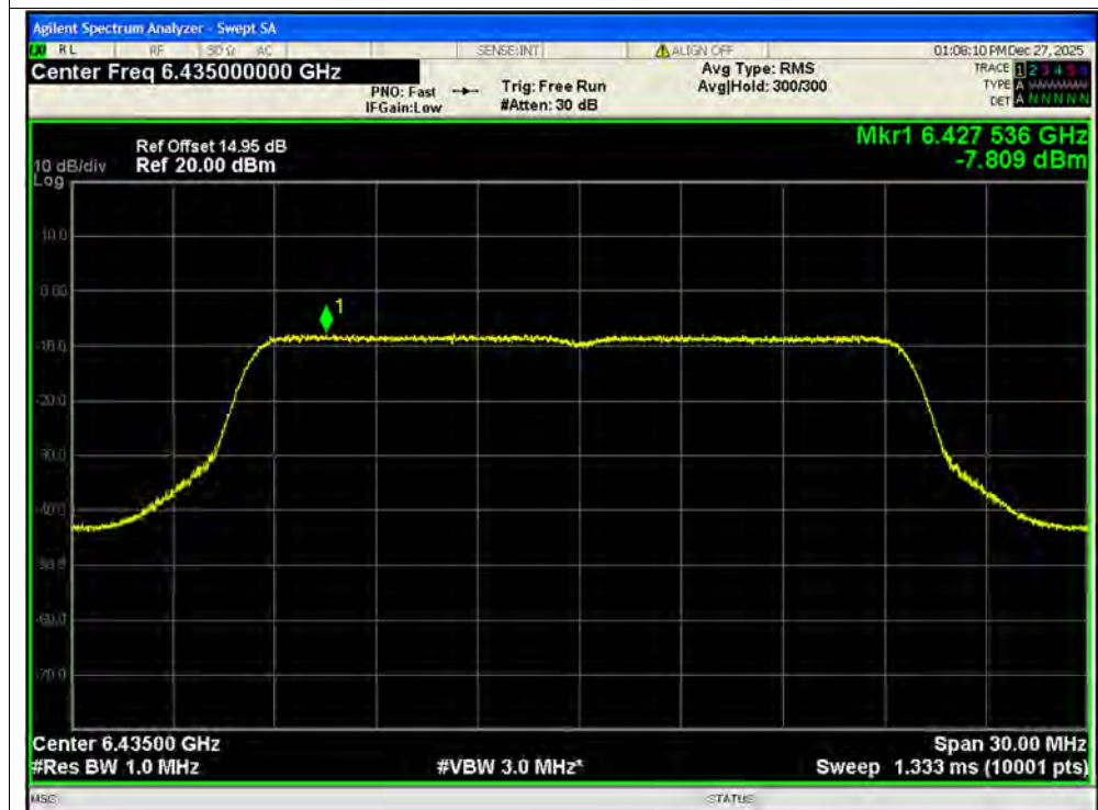
PSD NVNT ax20 6435MHz Ant2 SISO
