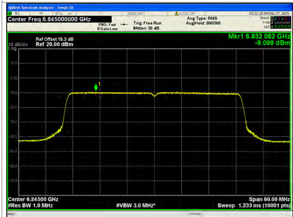
PSD NVNT ax40 6845MHz Ant2 MIMO
