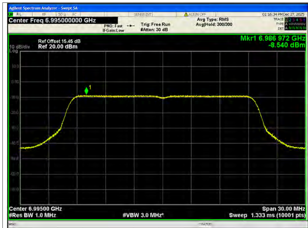
PSD NVNT ax20 6995MHz Ant2 SISO
