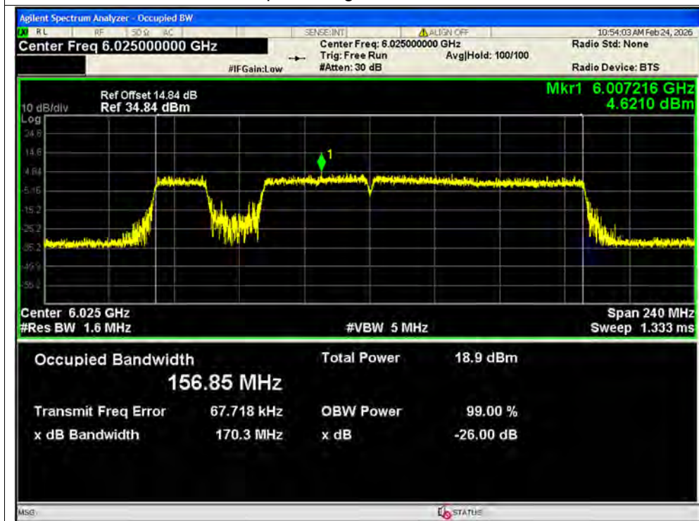
OBW NVNT be160 puncturing 20 MRU2 6025MHz Ant2 SISO
