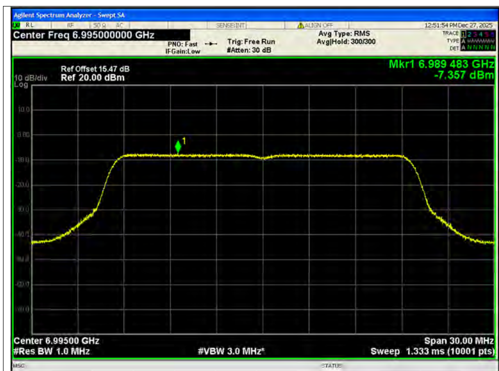
PSD NVNT be20 6995MHz Ant1 SISO
