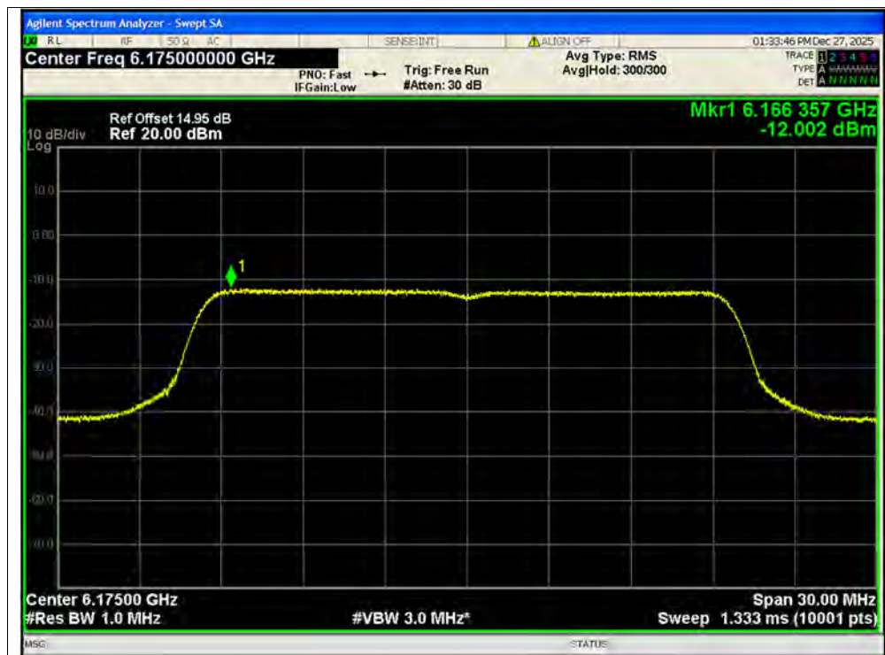
PSD NVNT ax20 6175MHz Ant1 MIMO
