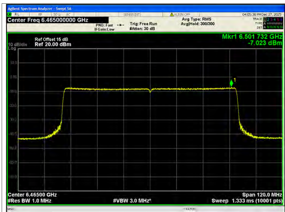
PSD NVNT ax80 6465MHz Ant2 SISO
