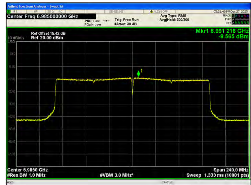
PSD NVNT ax160 6985MHz Ant2 SISO
