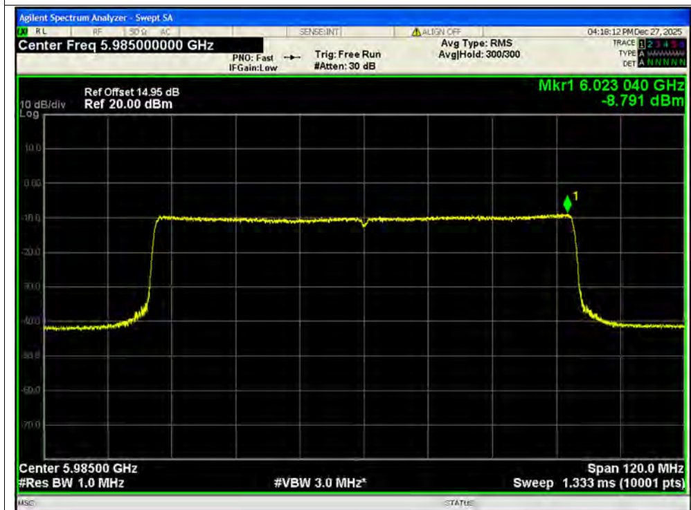
PSD NVNT ax80 5985MHz Ant2 MIMO
