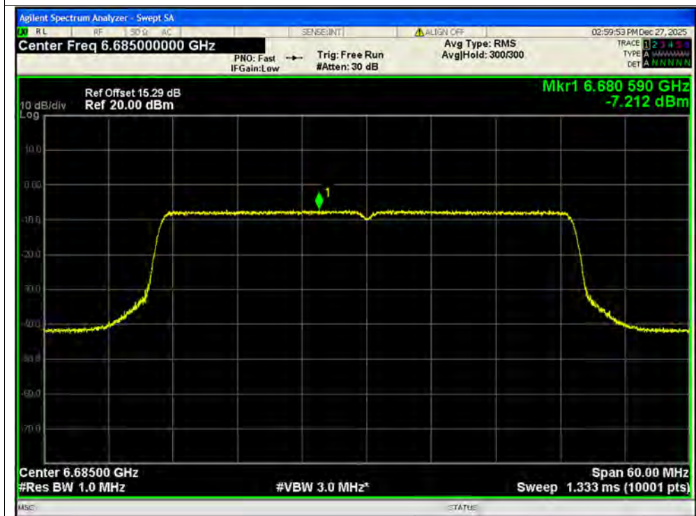
PSD NVNT ax40 6685MHz Ant2 SISO
