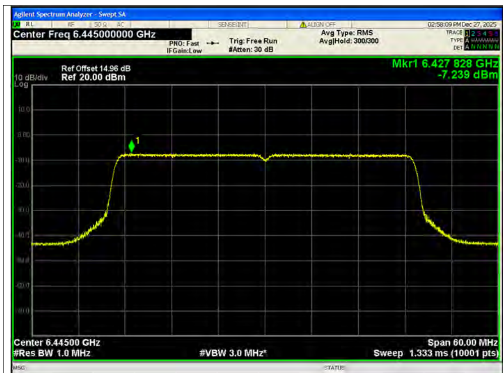
PSD NVNT ax40 6445MHz Ant2 SISO
