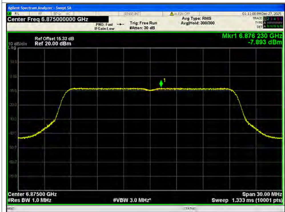
PSD NVNT ax20 6875MHz Ant2 SISO
