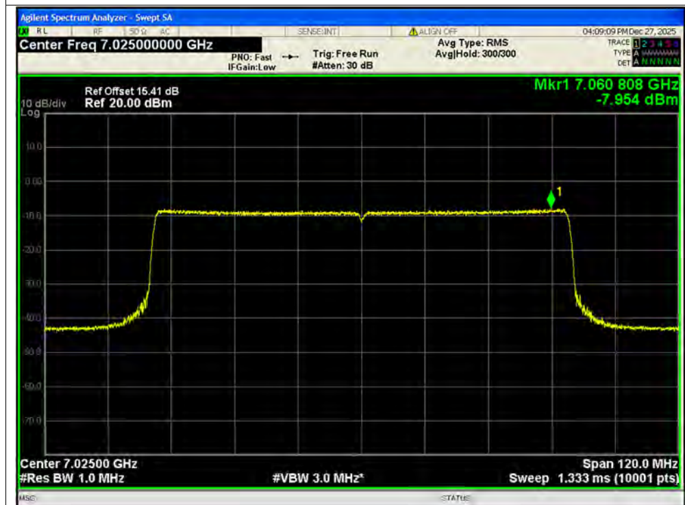
PSD NVNT ax80 7025MHz Ant2 SISO
