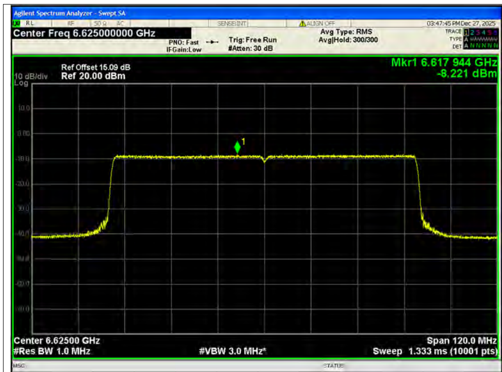
PSD NVNT ax80 6625MHz Ant1 SISO
