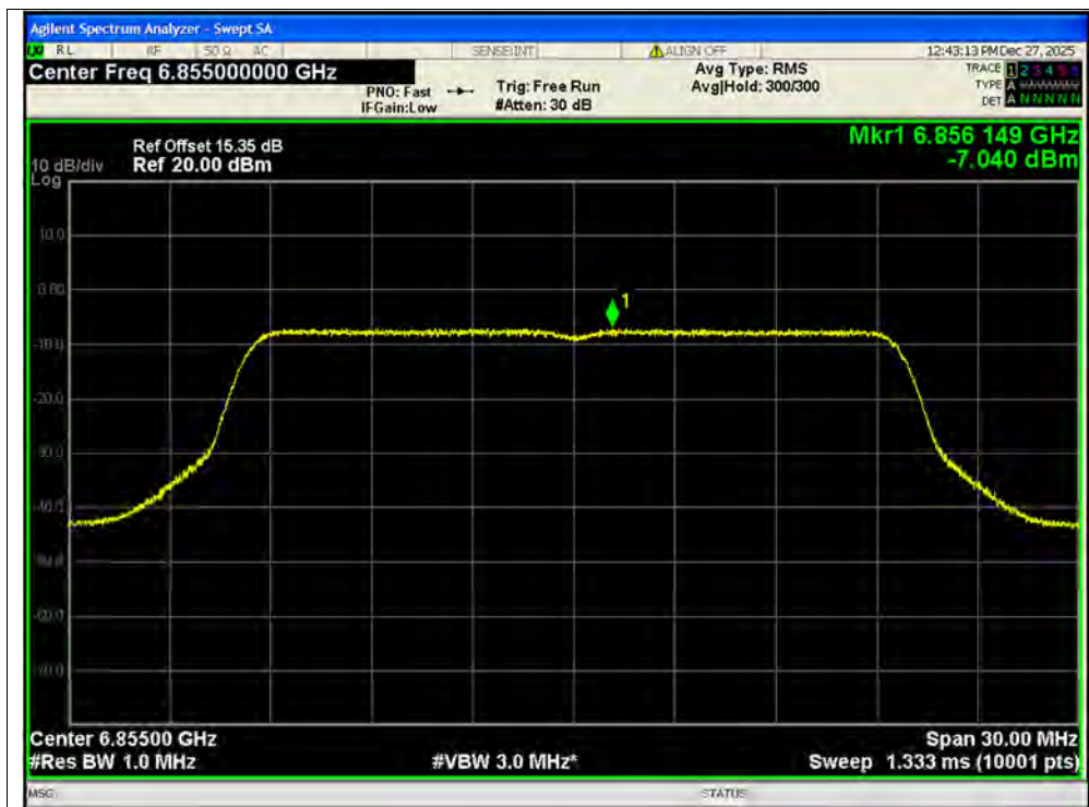
PSD NVNT ax20 6855MHz Ant1 SISO
