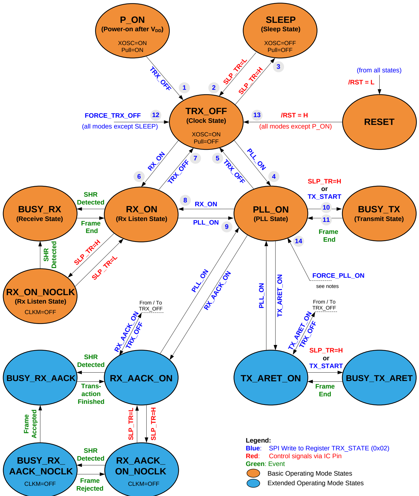
Figure 7-10. Extended Operating Mode State Diagram.
